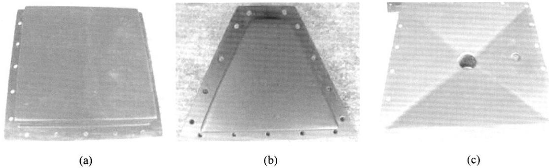
**Fig. 15.** Reactor walls coated with new coatings in pilot FGD system for accelerated testing of coating deterioration. (a) Side wall, (b) Hood bottom, (c) Drain bottom.
