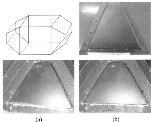
**Fig. 21.** Result in pilot FGD plant test of FLC-3 (graphite added, (a) 300 hours passed (b) 400 hours passed)
