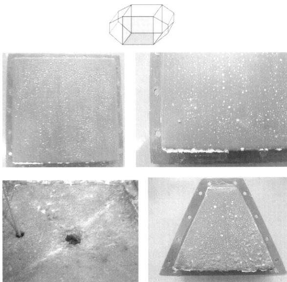
**Fig. 18.** Results in pilot FGD plant test of FLC-1 coating (Thickness = 25~30 $\mu$ m, 250 hours)
