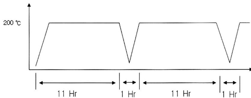
**Fig. 16.** Spraying condition of 20% sulphuric acid in pilot FGD system.
