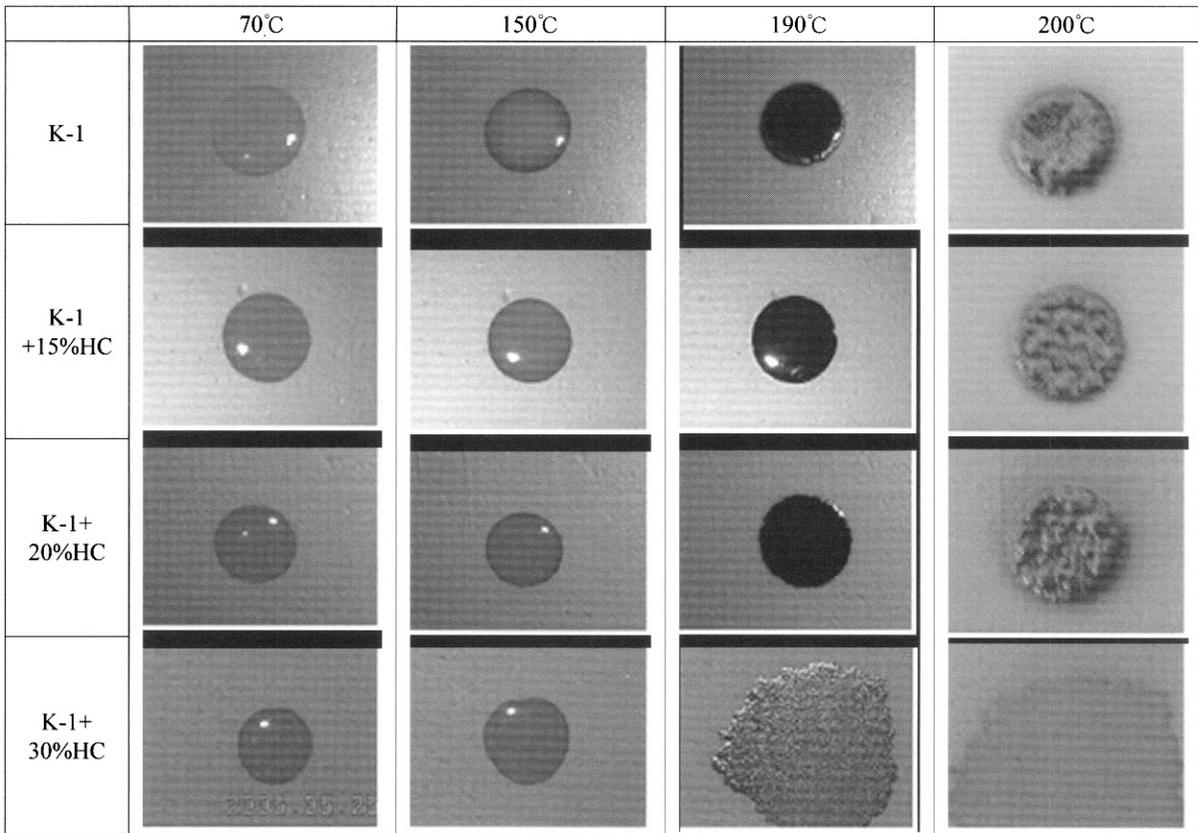
**Fig. 11.** The H<sub>2</sub>SO<sub>4</sub>(20%, up to 200°C)dropping test results of various newly developed epoxy Novolac coating materials varying with HC concentration.
