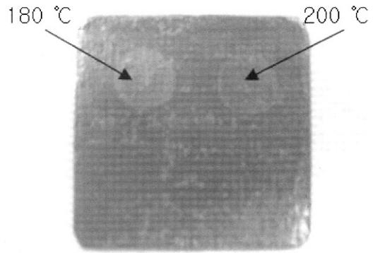
**Fig. 13. Coating surface of fluorine composite coating(FLC-1) after acid dropping test in high temperature.**
