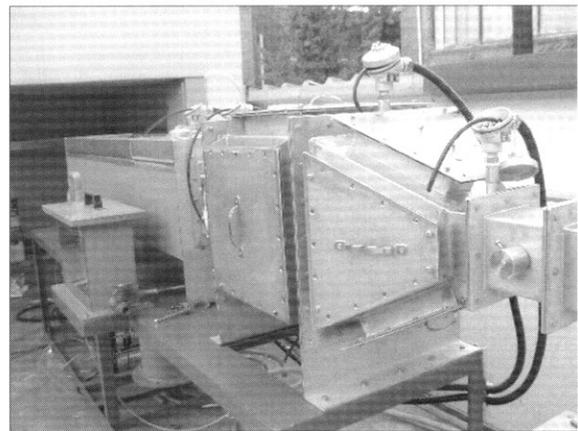
**Fig. 14. Pilot FGD system for accelerated testing of coating deterioration.**
