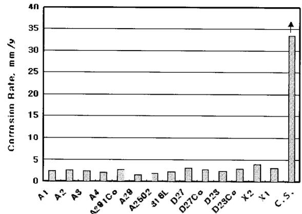
Fig. 4. Corrosion rates of several metallic coupons in FGD system
