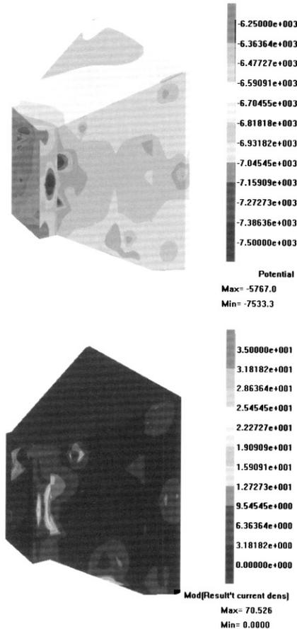
Fig. 6. Simulation results of CP system in FGD system
