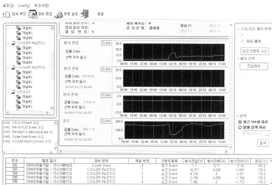
Fig. 5. Monitoring and controlling software of CP system installed in the FGD system
