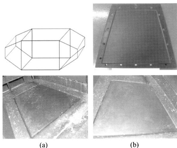
**Fig. 20.** Result in pilot FGD plant test of FLC-2 (carbon added, (a) 300 hours passed (b) 400 hours passed)
