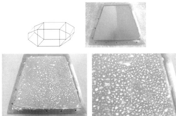
**Fig. 19.** Result in pilot FGD plant test of FRC-1 & FLC-1 (Thickness = 25~30 $\mu$ m, 250 hours)
