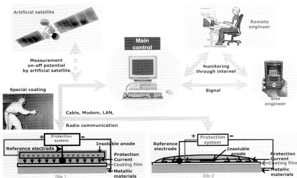
Fig. 3. Schematic diagram of CP system
