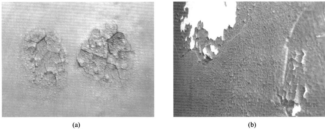
**Fig. 17.** Result in pilot FGD plant test of epoxy Novolac coating((a) pilot FGD, (b) real FGD plant)
