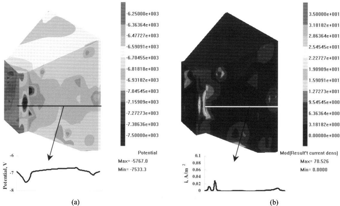
Fig. 10. Simulation result for cathodically protected area of outlet hood which it was coated ; (a) Protection potential, (b) Protection current density
