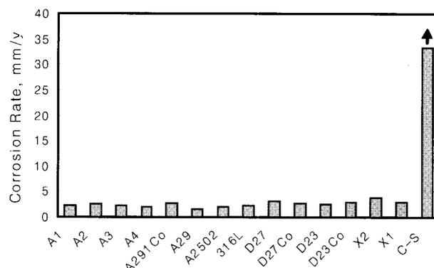
Fig. 3. Corrosion rates of several metallic coupons in the FGD system
