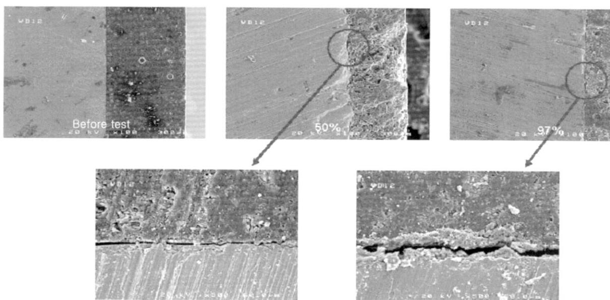
Fig. 4. Delamination between metal and coating with variation of acid concentrations
