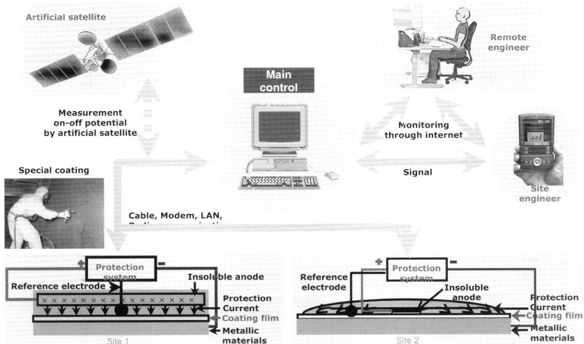
**Fig. 8. Schematic diagram of CP system<sup>1)</sup>**
