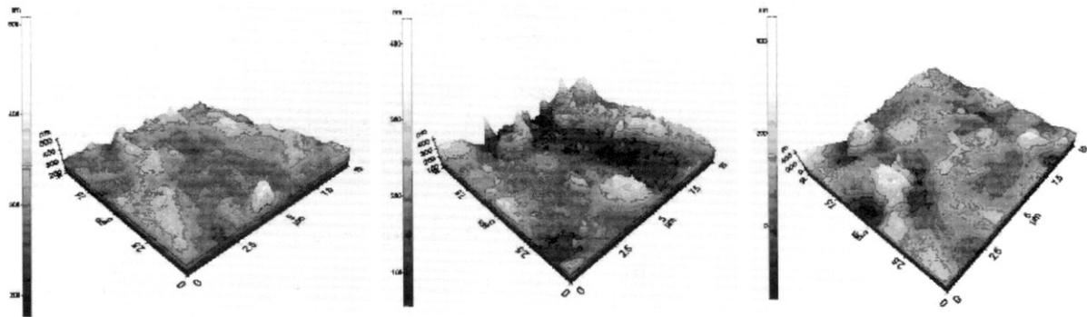
**Fig. 6.** Surface analysis of the coatings damaged by sulfuric acid (AFM) - 3D
