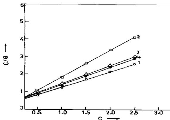
Fig. 2. Langmuir adsorption isotherm plot for the adsorption of various concentrations natural product extracts on mild steel in 1M HCl solution
