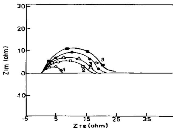
**Fig. 5.** Impedance diagrams for mild steel in 1M HCl solution containing various concentrations of jackfruit seed extract
