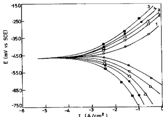
**Fig. 4.** Potentiodynamic polarization curves for mild steel in 1M HCl solution containing various concentrations of henna leaves extract
