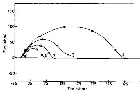
**Fig. 6.** Impedance diagrams for mild steel in 1M HCl solution containing various concentrations of henna leaves extract (1) Blank (2) 1.0 ml (3) 1.5 ml (4) 2.0 ml (5) 2.5 ml
