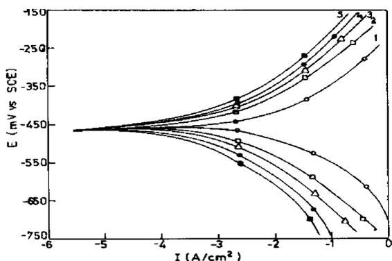
**Fig. 3.** Potentiodynamic polarization curves for mild steel in 1M HCl solution containing various concentrations of jackfruit seed extract
