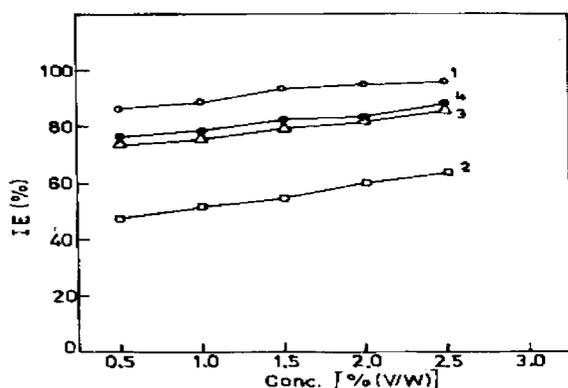
Fig. 1. Plot of inhibition efficiency with various concentrations of natural product extracts for corrosion of mild steel in 1M HCl solution
