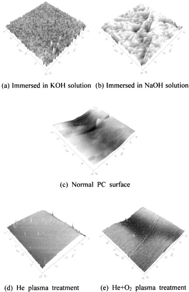
Fig. 3. 3-D images of prepared PC's surface.
