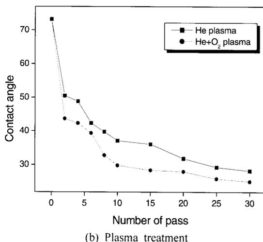
**Fig. 2.** Contact angle of PC surface by etching and plasma treatment.
