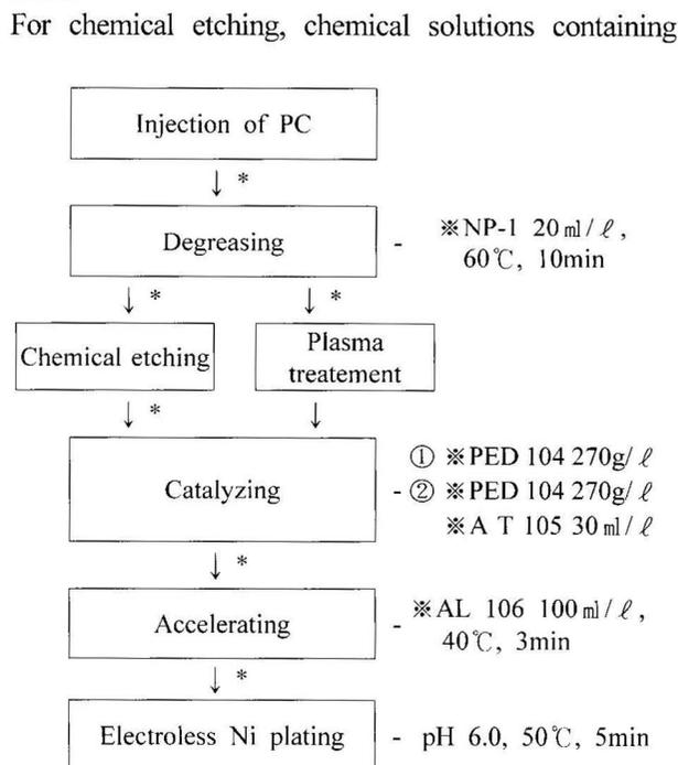
**Fig. 1.** Schematic diagram of Ni plating process.
