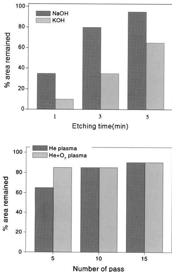
Fig. 7. Adhesion of plating layer on PC by tape test after boiling test.
