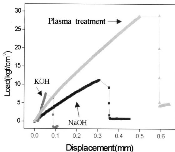
Fig. 6. Adhesive strength of plating layer on PC by pull test.
