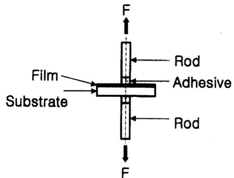
Fig. 5. Schematic diagram of pull test.
