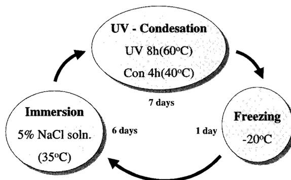
Fig. 1. Method for deterioration of specimens
