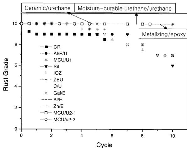
Fig. 4. Rust grades by ASTM D 610
