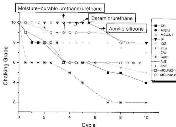
**Fig. 2.** Chalking grades by ASTM D 4214
