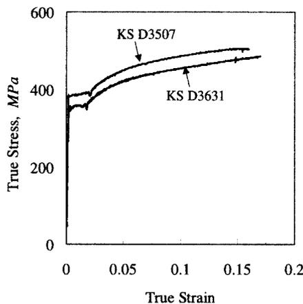
Fig. 4. True stress-strain curves for KS D3507 and KS D3631
