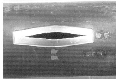
Fig. 2. Picture of (a) burst test equipment and (b) specimen 3631C after test
