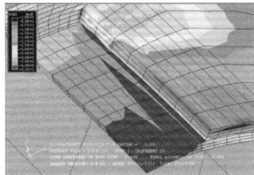
Fig. 5. Contour plot of von Mises stress at the corroded area
