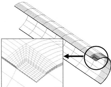
Fig. 3. A typical finite element mesh used for burst test simulation
