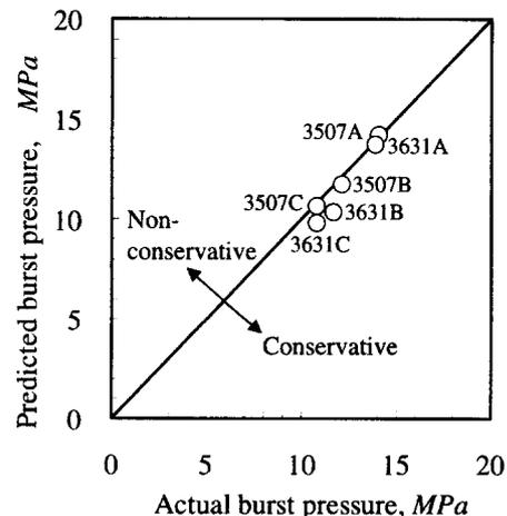
Fig. 6. Comparison between actual burst pressure and burst pressure predicted from finite element simulation
