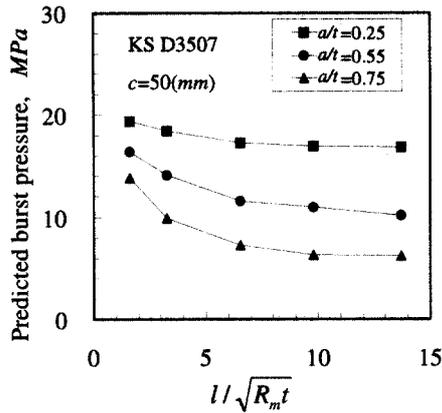
Fig. 7. Burst pressure predicted from finite element analysis for various defect shape
