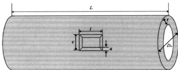
Fig. 1. A schematic illustration of burst test specimen
