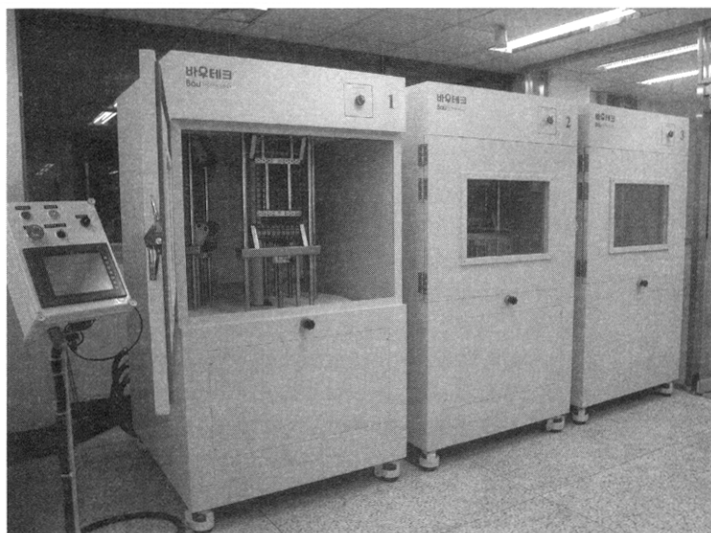
Fig. 2. Accelerated creep test equipment
