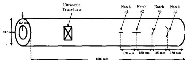
Fig. 3. Configuration of the artificial notches in a feeder pipe.
