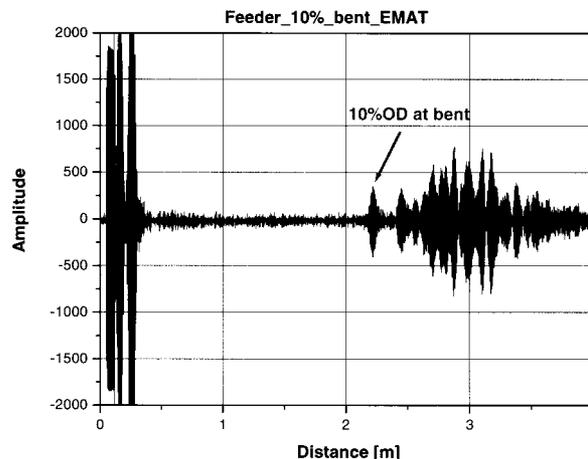
(b) Signal from a notch of 10% of the wall thickness of the bent pipe.
