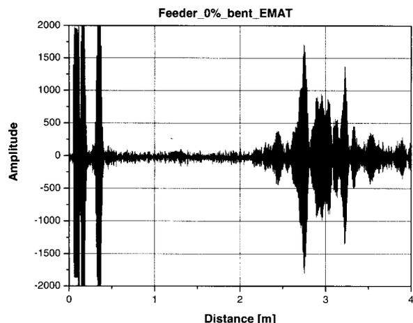
(a) Signal from a bent pipe with no defect.
