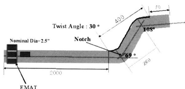
Fig. 6. Configuration of the guided wave inspection of the artificial notches in the Feeder pipe.
