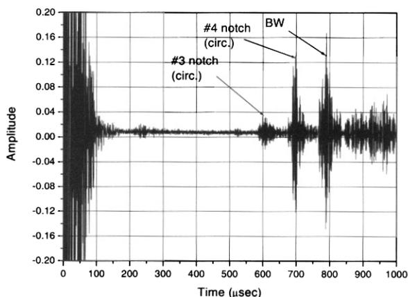
(a) Guided wave signal from a straight pipe with 4 notches ( $f=500\text{ kHz}$ ,  $F(m,2)$  mode)
