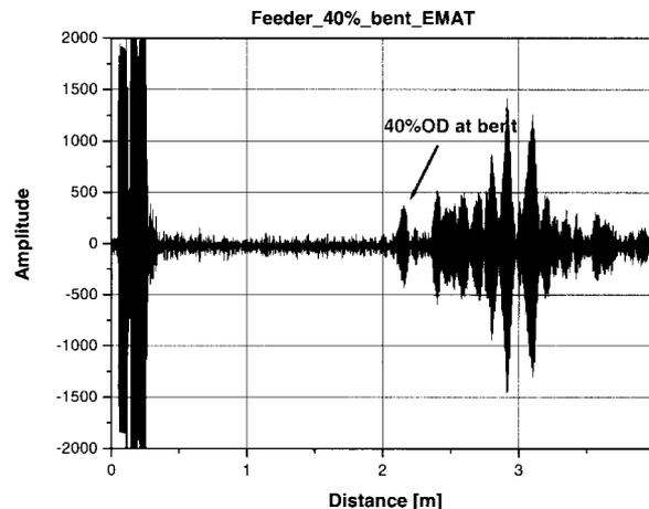
(b) Signal from a notch of 40% of the wall thickness of the bent pipe.
