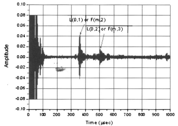
(a) Signal received from the end of a feeder pipe ( $f = 500$  kHz, metal path = 0.5m).
