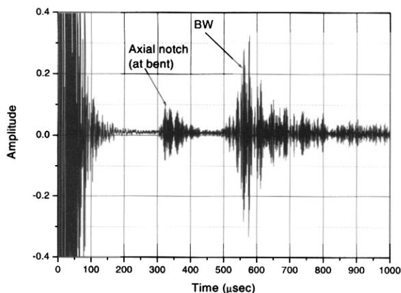
(b) Guided wave signal from a bent pipe with a notch ( $f=500\text{ kHz}$ ,  $F(m,2)$  mode)
