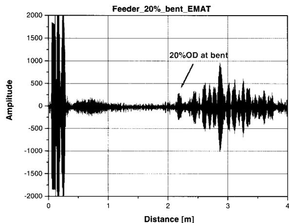
(c) Signal from a notch of 20% of the wall thickness of the bent pipe.
