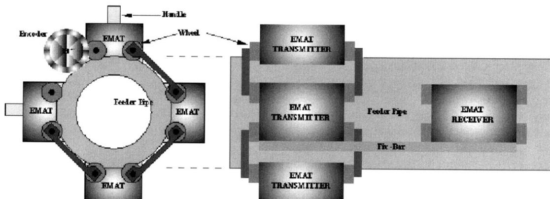
Fig. 5. An array of EMATs for the generation and reception of the torsional guided wave.
