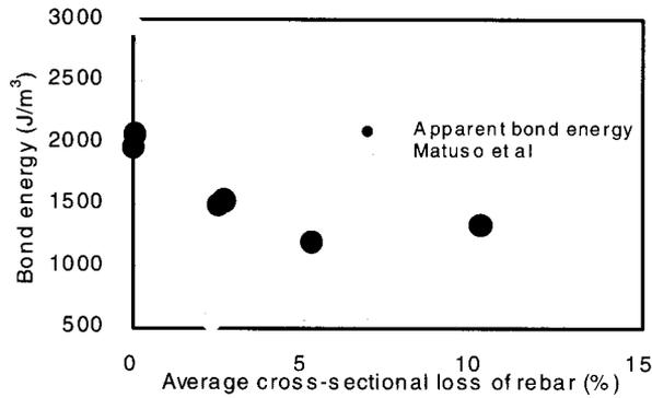
Fig. 13. Bond fracture energy
