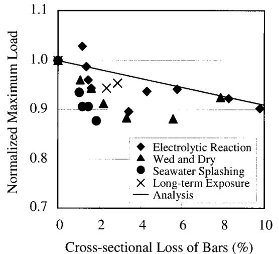
Fig. 4. Load-carrying capacity of the beam
