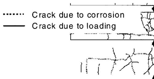
Fig. 5. Crack formation at  $3\delta_y$
