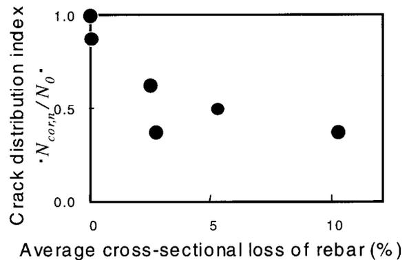
Fig. 11. Crack distribution index
