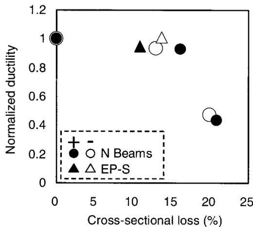
Fig. 7. Ductility by corrosion of main bars
