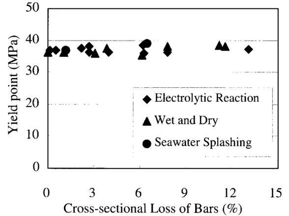
Fig. 3. Yield point of corroded bars
