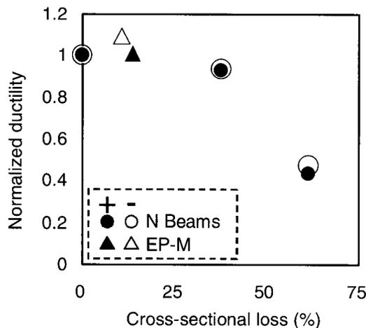
Fig. 8. Ductility by corrosion of stirrups
