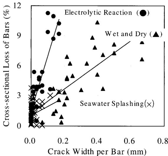
Fig. 2. Cross sectional loss vs crack width
