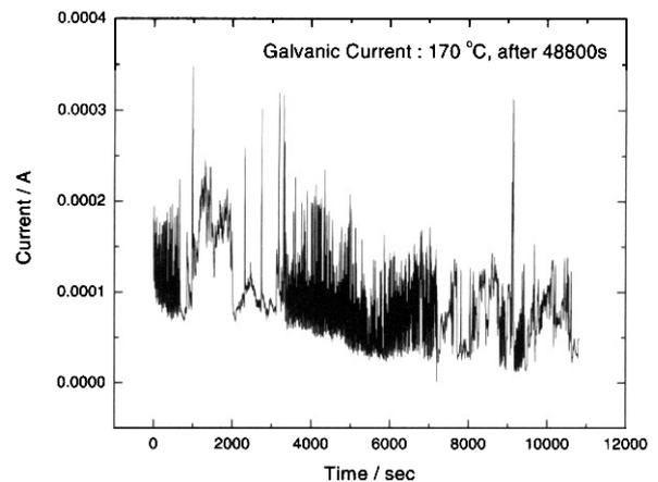
Fig. 2. Typical current transient obtained during galvanic coupling between 1018 carbon steel and alloy 600 in the aqueous solution containing 2000 ppm boron and 3.5 ppm lithium.
