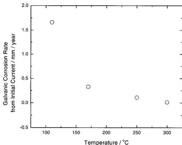
Fig. 7. Galvanic corrosion rate obtained from initial galvanic current as a function of operating temperature in the range of 110 to 300 °C in the aqueous solution containing 2000 ppm boron and 3.5 ppm lithium.
