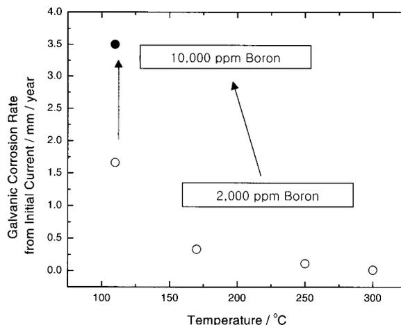
Fig. 8. Plot of galvanic corrosion rate against boron concentration of 2000 ppm(O) and 10000 ppm(l) in the solution.
