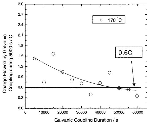
**Fig. 3.** Plot of charge passed per each 5000 s during galvanic coupling between 1018 carbon steel and alloy 600 against galvanic coupling duration at 170 °C in the aqueous solution containing 2000 ppm boron and 3.5 ppm lithium.
