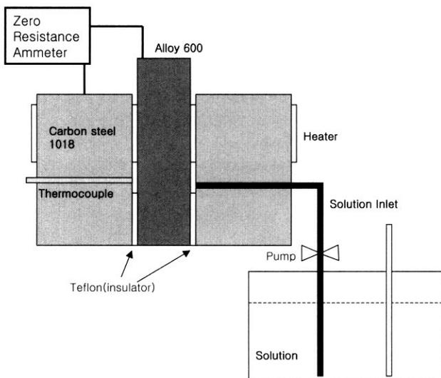
Fig. 1. Schematic diagram showing experimental apparatus.
