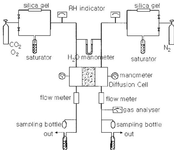
Fig. 1. Gas diffusion measurement system
