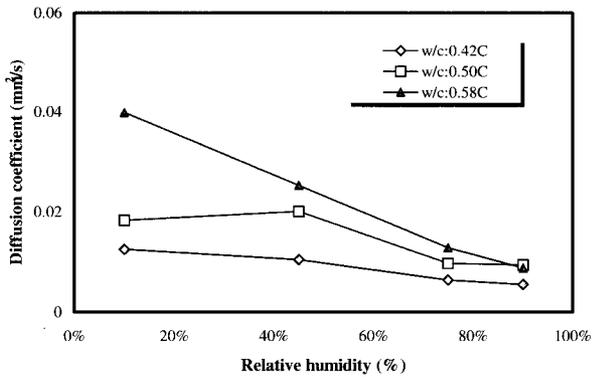
Fig. 6. Variation of diffusion coefficient according to relative humidity
