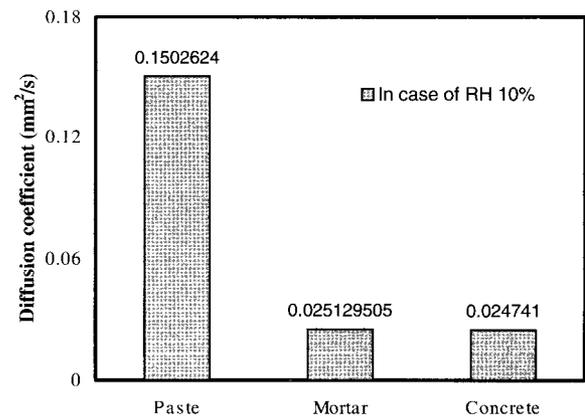
Fig. 9. Diffusion coefficient of carbon dioxide in case of 10% relative humidity
