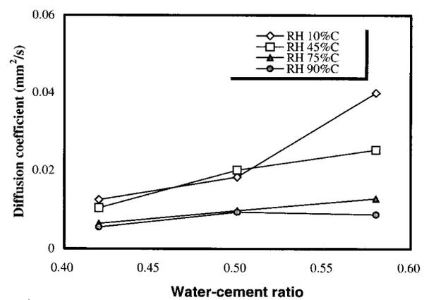
(b) In case of carbonated concrete
