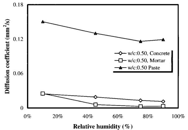
Fig. 8. Variation of diffusion coefficient according to RH with various materials
