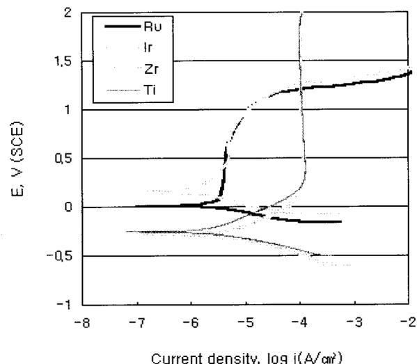
Fig. 1. Anodic polarization curves of single component coating (Ru, Ir, Zr coating on the Ti substrate) and Ti substrate in 1M H<sub>2</sub>SO<sub>4</sub> solution at 25°C
