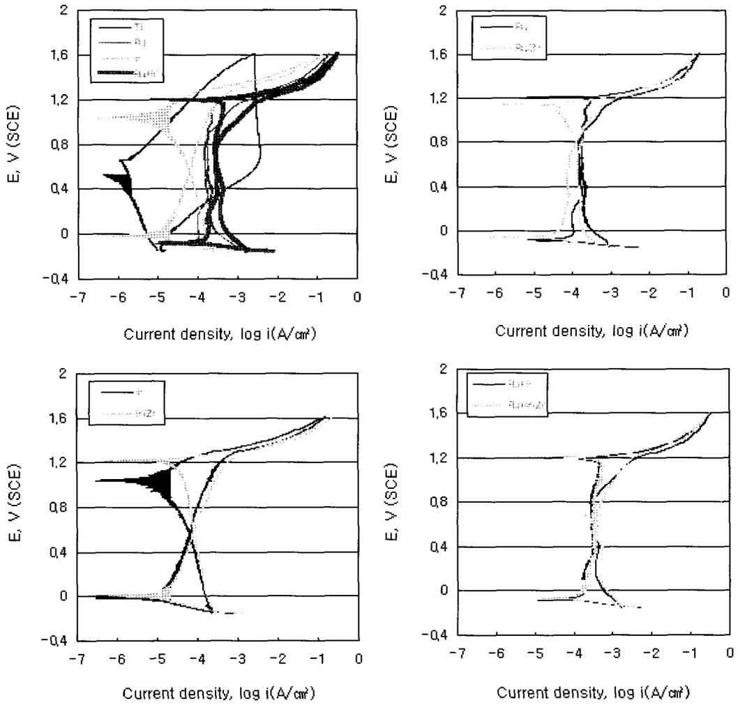
Fig. 3. Cyclic polarization of Ru or Ir or Zr coating on the Ti substrate and Ti substrate in 0.5M  $H_2SO_4$  solution at 25°C
