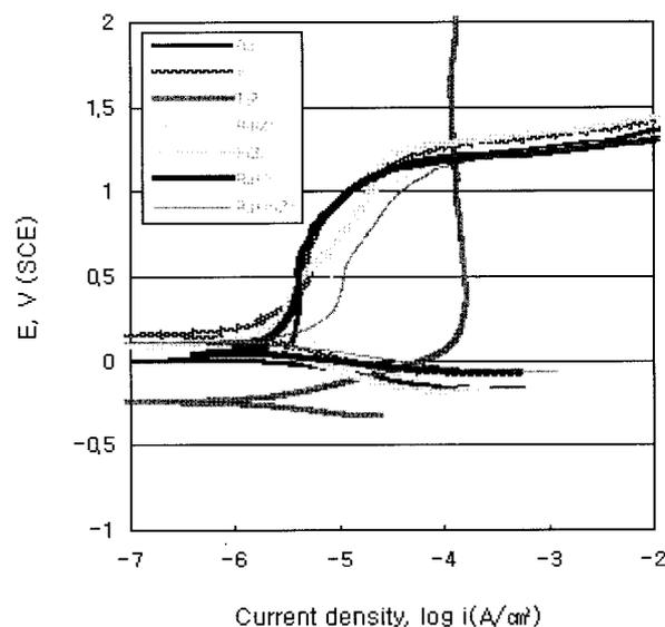
Fig. 2. Anodic polarization curves of Ru or Ir or Zr coating on the Ti substrate and Ti substrate in 1M H<sub>2</sub>SO<sub>4</sub> solution at 25°C
