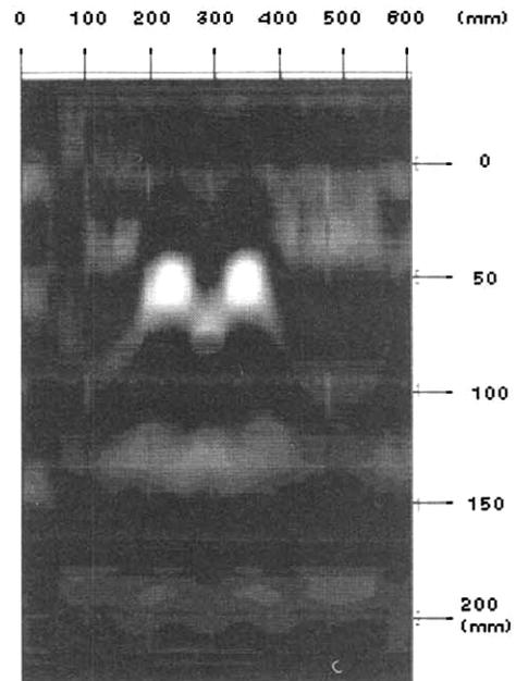
Fig. 6. Radar imaging with improved signal processing scheme (horizontal spacing is 12 cm).
