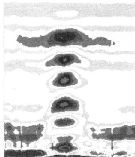
Fig. 7. Output of radar measurements (delamination depth is 25 mm)
