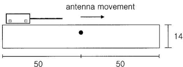
Fig. 1. Dimensions of concrete specimen for the radar measurements in cm. Locating the bar is much easier compared to Fig. 2.
