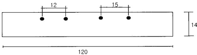
Fig. 4. Dimensions of concrete specimen for the radar measurements in cm.
