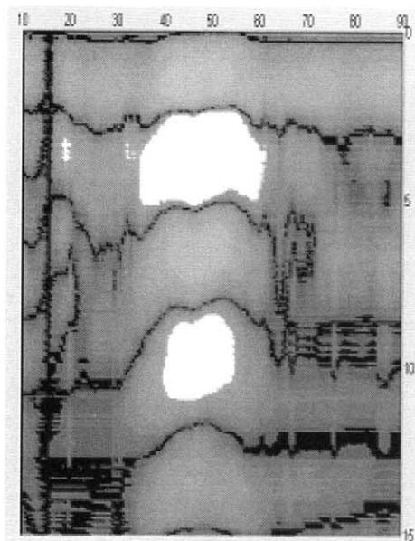
Fig. 8. Radar imaging with improved signal processing scheme (delamination depth is 25 mm).
