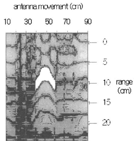
Fig. 3. Radar imaging with improved signal processing scheme.
