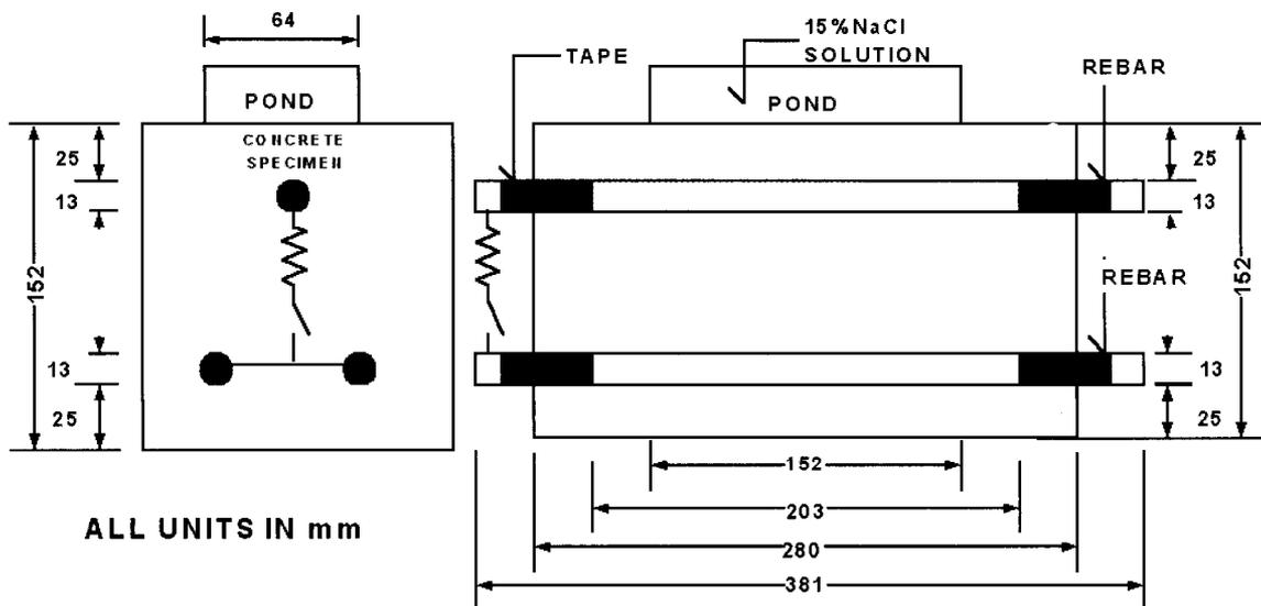
**Fig. 1. Geometry of the classical G109 specimen**
