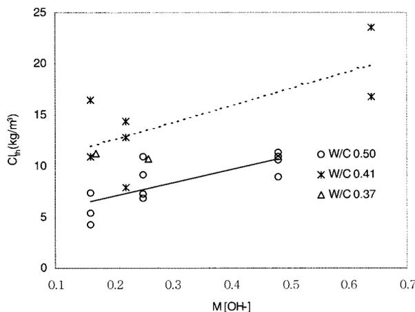
Fig. 9. The change of chloride thresholds ( $Cl_{th}$ ) with respect to  $M[OH^-]$ .
