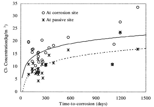
Fig. 8. Chloride thresholds ( $Cl_{th}$ ) with respect to time-to-corrosion ( $T_i$ ).
