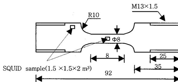
Fig. 2. Configuration of fatigue specimen and extraction position of HTS SQUID sample.
