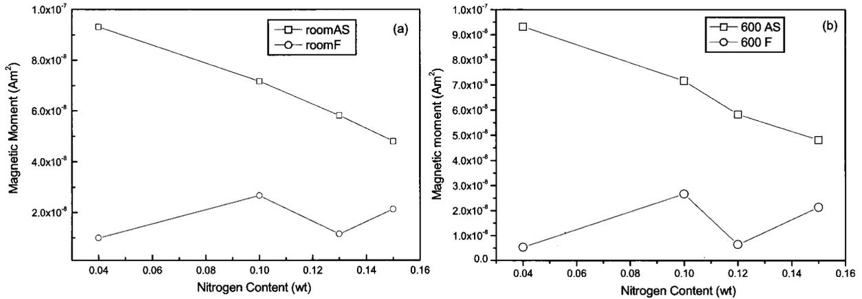
Fig. 3. Change of magnetic moment with nitrogen content (a) tested at room temperature (b) tested at 600 °C
