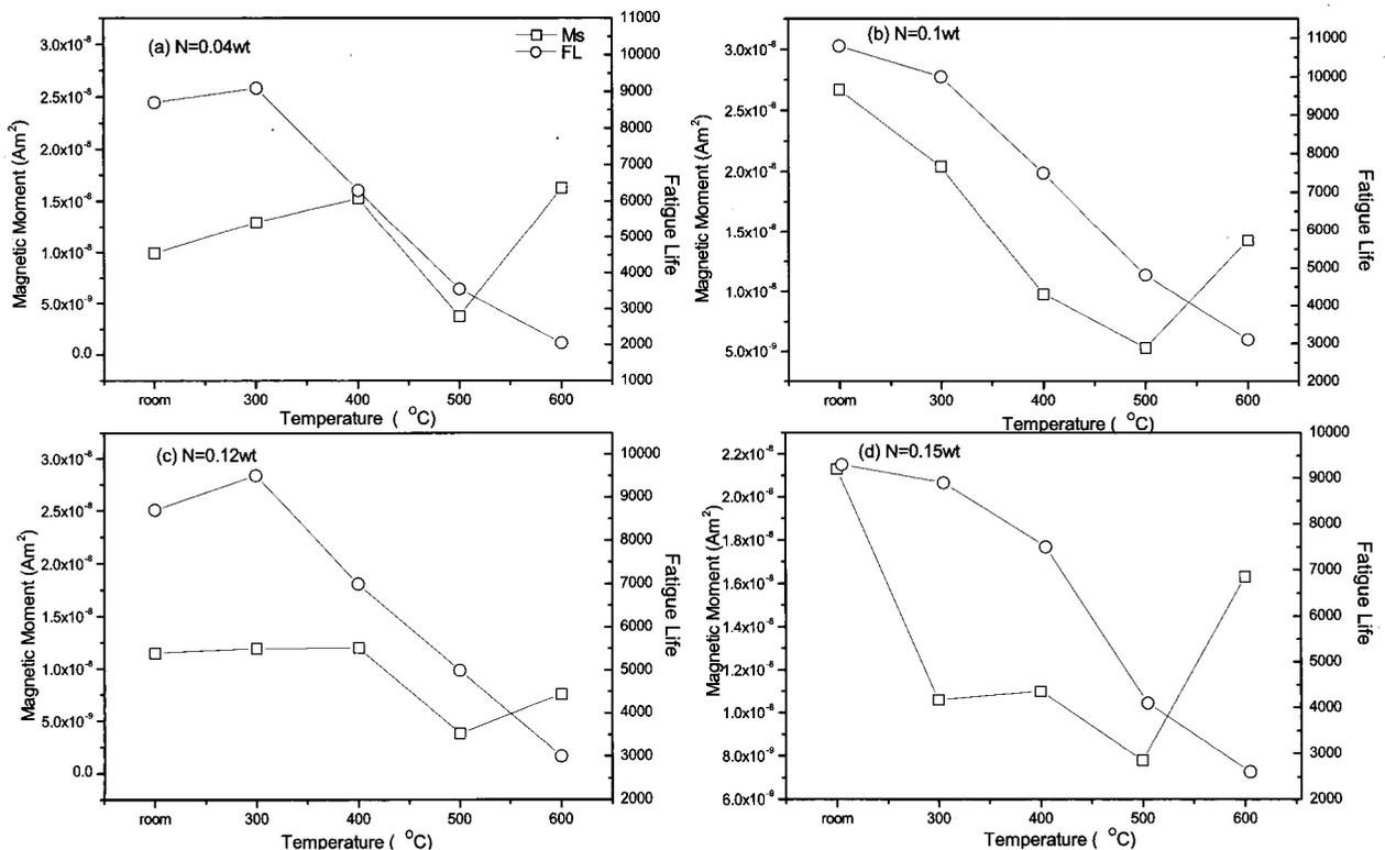
Fig. 4. Temperature dependence of magnetic moment and fatigue life with nitrogen contents. (a) nitrogen content of 0.04wt, (b) 0.1 wt, (c) 0.12 wt, (d) 0.15 wt.
