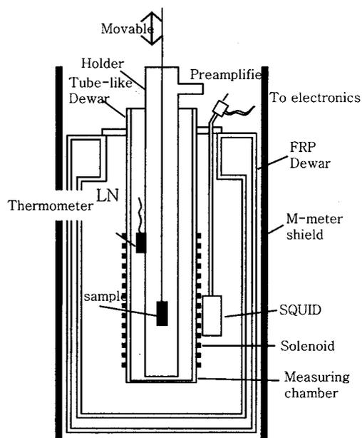
Fig. 1. Construction of HTS RF SQUID-based Susceptometer.
