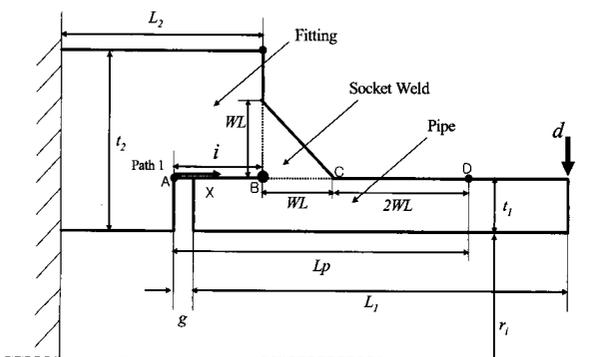
Fig. 1. Geometry of Socket Weld with Pipe and Fitting
