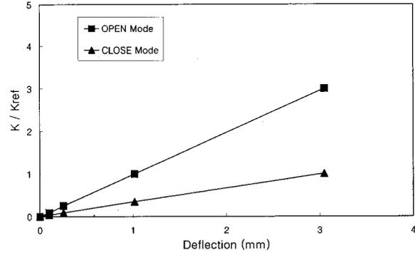
Fig. 4. Deflection Effect on Stress Intensity Factor( $K$ ) normalized as  $K_{ref} = 289$  MPa√(mm).
