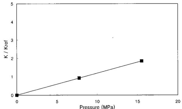
Fig. 5. Pressure Effect on Stress Intensity Factor( $K$ ) normalized as  $K_{ref} = 289$  MPa√(mm).
