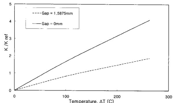
Fig. 8. Gap Effect on Stress Intensity Factor(K) normalized as  $K_{ref} = 289 \text{ MPa}\sqrt{\text{mm}}$  as a function of Temperature.
