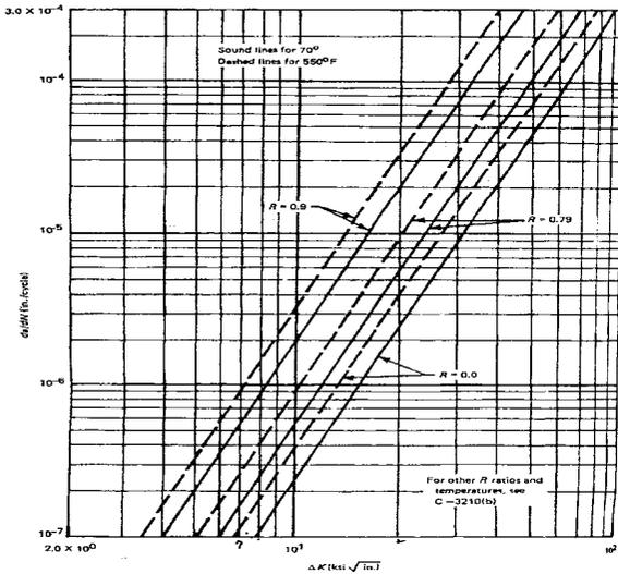
Fig. 3. Fatigue Crack Growth Curve for Stainless Steel
