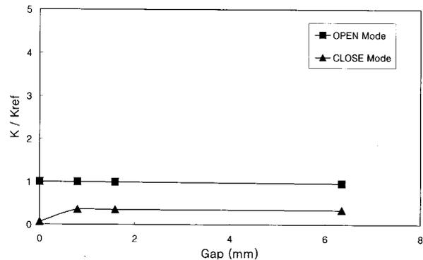
Fig. 7. Gap Effect on Stress Intensity Factor(K) normalized as  $K_{ref} = 289 \text{ MPa}\sqrt{\text{mm}}$  under Deflection Load.
