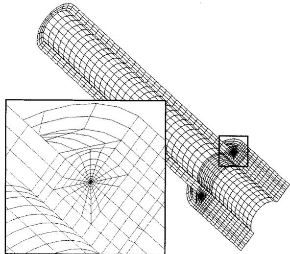
Fig. 2. 3 Dimensional FEM Modelling for Socket Weld Analysis
