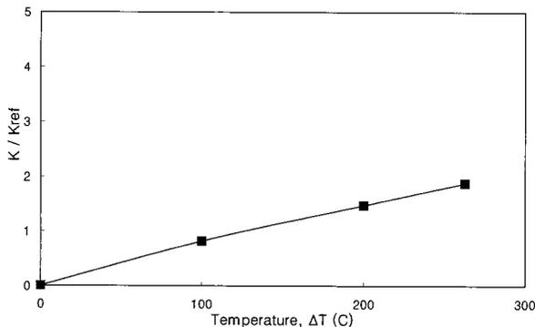
Fig. 6. Temperature Effect on Stress Intensity Factor(K) normalized as  $K_{ref} = 289 \text{ MPa}\sqrt{\text{mm}}$ .
