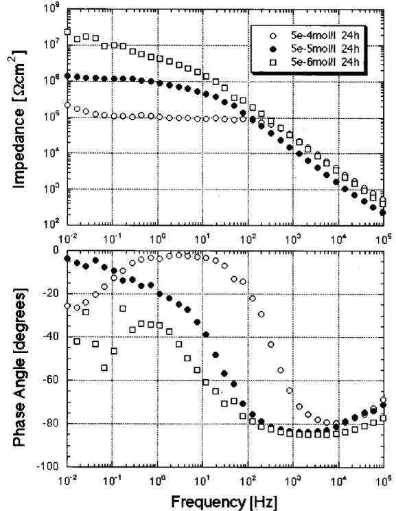
Fig. 5. Impedance behavior for TDK DVC ME tape after 24h immersion in H<sub>2</sub>SO<sub>4</sub> solution with different concentration.
