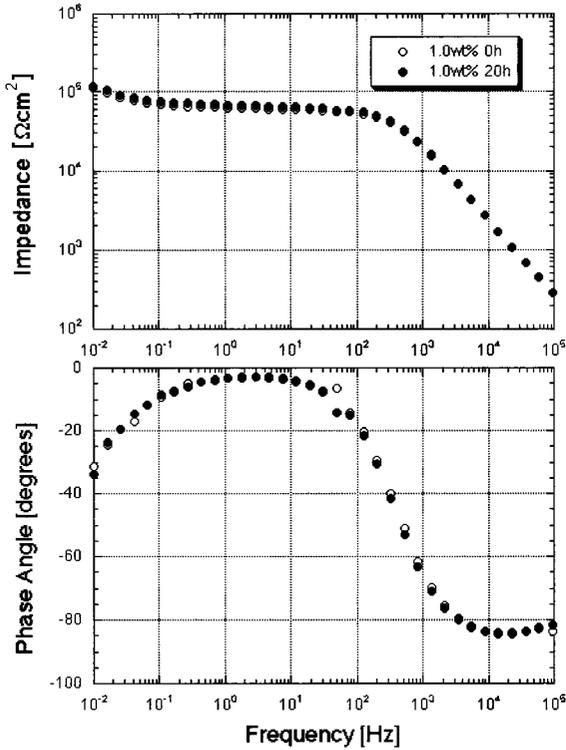
Fig. 1. Changes in impedance behavior for Hi8 mm TDK video tape in 1.0 wt% NaCl solution.
