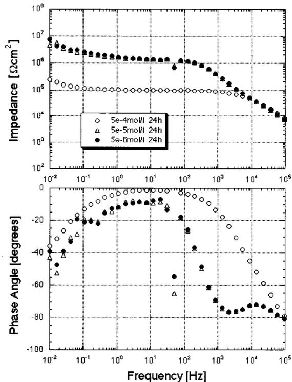
Fig. 4. Impedance behavior for Hi8 mm TDK video tape after 24h immersion in H<sub>2</sub>SO<sub>4</sub> solution with different concentration.
