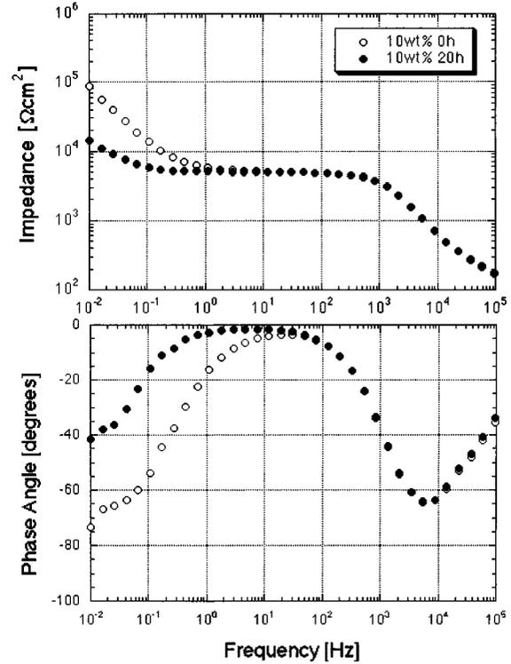
Fig. 2. Changes in impedance behavior for Hi8 mm TDK video tape in 10 wt% NaCl solution
