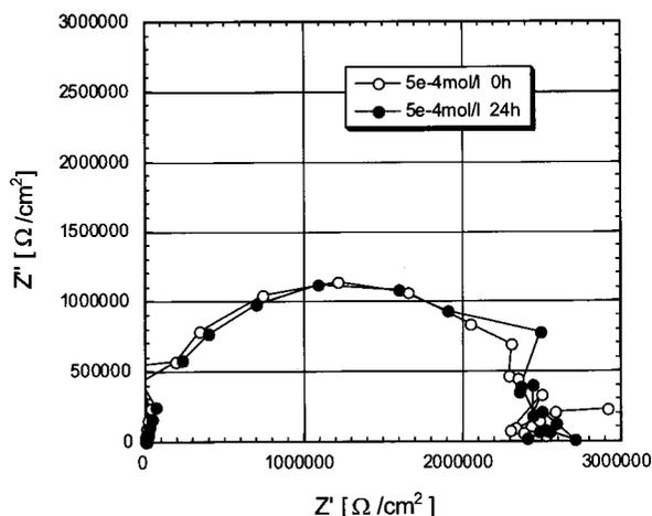
**Fig. 7.** Changes in impedance behavior for the backside TDK DVC ME tape with time in  $5 \times 10^{-4} \text{M}$   $\text{H}_2\text{SO}_4$  solution.
