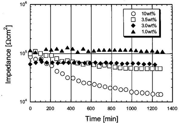
Fig. 3. Changes in impedance at 10 mHz for Hi8 mm TDK tape in NaCl solutions.
