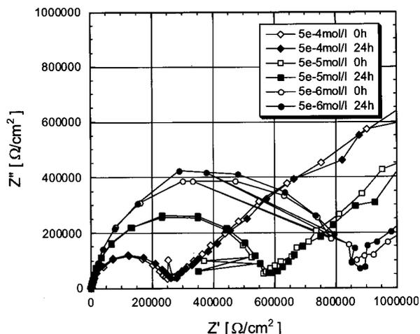
**Fig. 6.** Changes in impedance behavior for the backside of Hi-8 mm TDK ME tape with time in  $\text{H}_2\text{SO}_4$  solution with different concentration.
