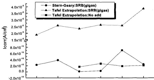
Fig. 6. Comparative analysis of corrosion current densities measured by Tafel and Stern-Geary methods for Mild, Normalized and TMCP steels in the presence and absence of the SRB *Desulfovibrio gigas* (KCTC 2483).
