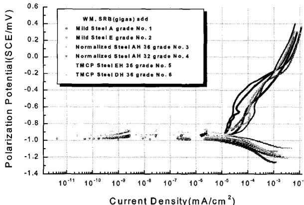
Fig. 4. Cathodic and anodic polarizations curves for various kinds
