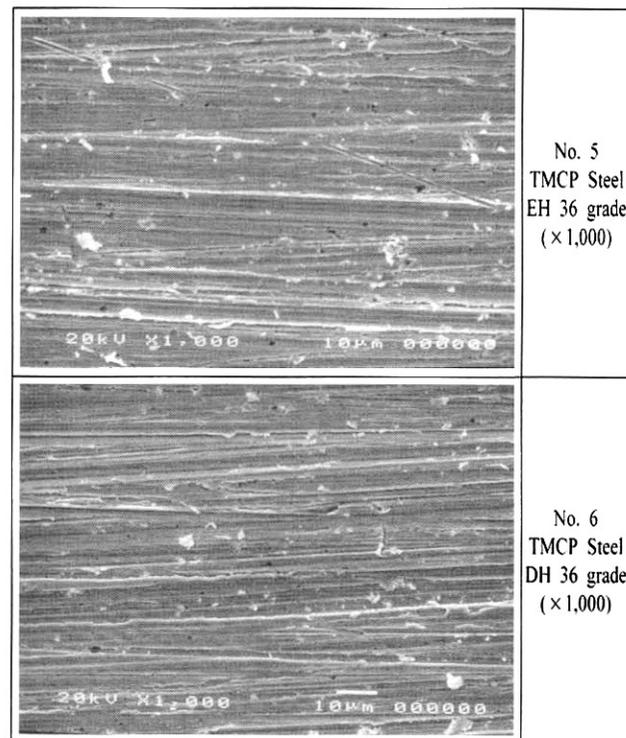
Plate 2. SEM photographs of polished surface for test specimens after 40 days without the SRB strain KMU-2 inoculation.
