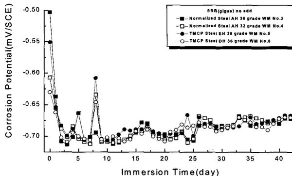
Fig. 3. Time course of corrosion potential in liquid medium without inoculation of the SRB *Desulfovibrio gigas* (KCTC 2483)
