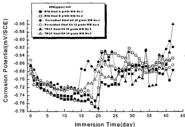
Fig. 2. Time course of corrosion potential in liquid medium
