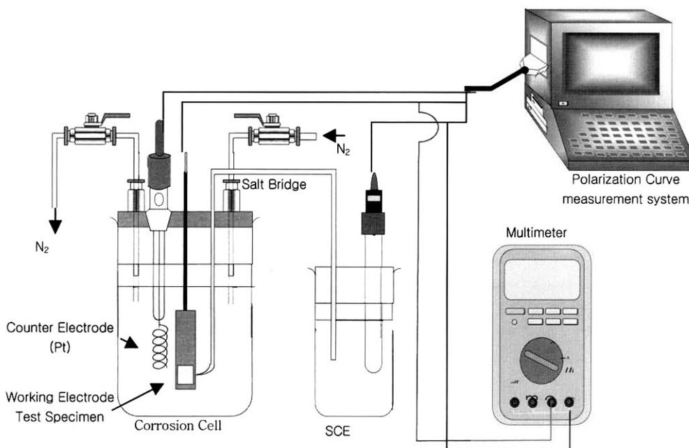
Fig. 1. Schematic diagram of the experimental apparatus for corrosion test
