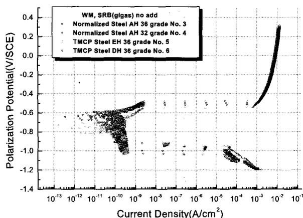
Fig. 5. Polarization curves of Normalized and TMCP steels without the inoculation of *Desulfovibrio gigas* (KCTC 2483)
