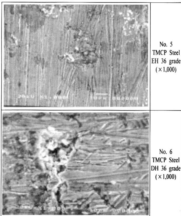
Plate 1. SEM photographs of polished surface for test specimens after 40 days' incubation with the SRB strain KMU-2 isolated from a crude oil sample
