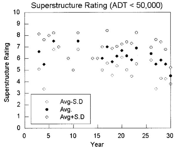
Fig. 10. Condition Rating of Steel Girders (ADT < 50,000)
