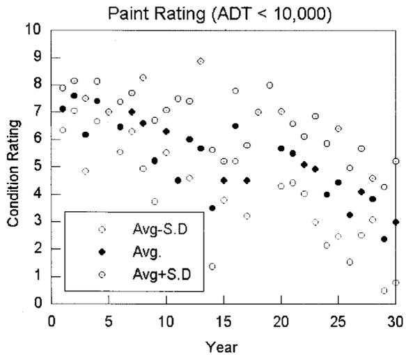
Fig. 3. Paint Condition Rating (ADT <10,000)
