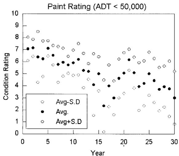
Fig. 4. Paint Condition Rating (ADT <50,000)
