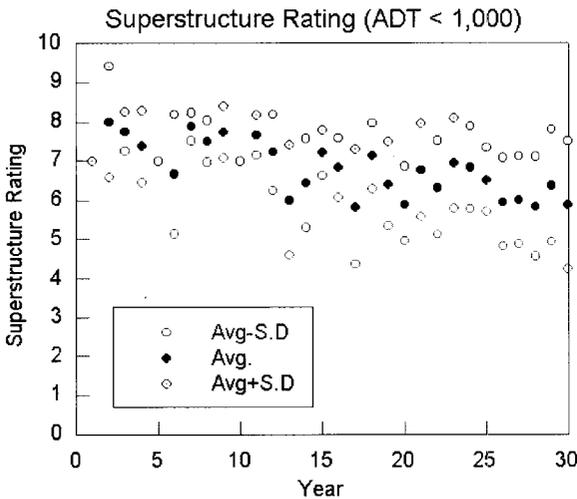
Fig. 8. Condition Rating of Steel Girders (ADT < 1,000)
