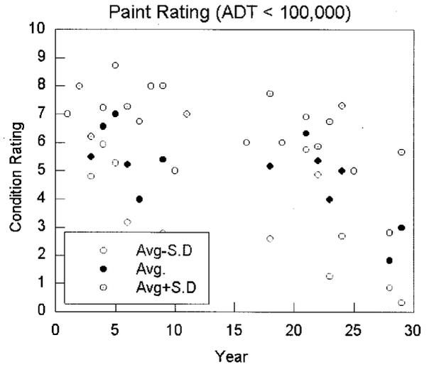
Fig. 5. Paint Condition Rating (ADT <100,000)
