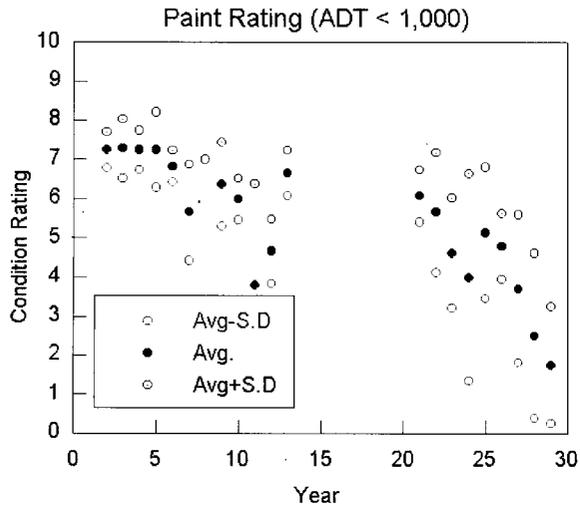
Fig. 2. Paint Condition Rating (ADT <1,000)
