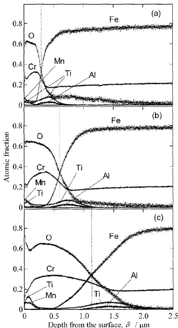
**Fig. 9.** Compositional depth profiles by GD-OES of Fe-19Cr-0.2Ti alloys oxidized for (a) 300 s, (b) 600 s, (c) 1800 s in 16.5 kPa  $O_2$  bal.  $N_2$  atmosphere.
