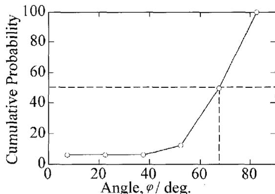
Fig. 7. Cumulative probability of the angle between major axis of oxide grains and specimen surface.
