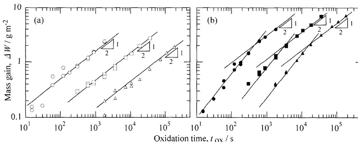
**Fig. 1.** Changes in mass gain with oxidation time, for (a) Fe-19Cr, (b) Fe-19Cr-0.2Ti alloys oxidized in 16.5 kPa O<sub>2</sub> balanced N<sub>2</sub> atmosphere at 1173 K (triangle), 1273 K (square), and 1373 K (circle).
