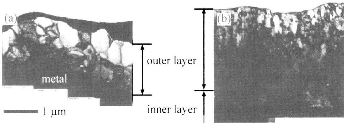
Fig. 6. TEM photographs of the oxide films formed on (a) Fe-19Cr and (b) Fe-19Cr-0.2 Ti alloys oxidized at 1273 K for 10.8 ks.
