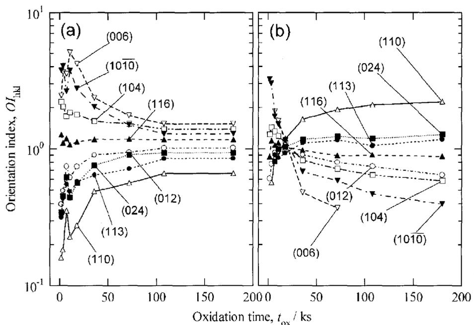
Fig. 4. Orientation indices of corundum type (Fe, Cr)<sub>2</sub>O<sub>3</sub> oxide formed on (a) Fe-19Cr and (b) Fe-19Cr-0.2Ti alloys at 1173 K.
