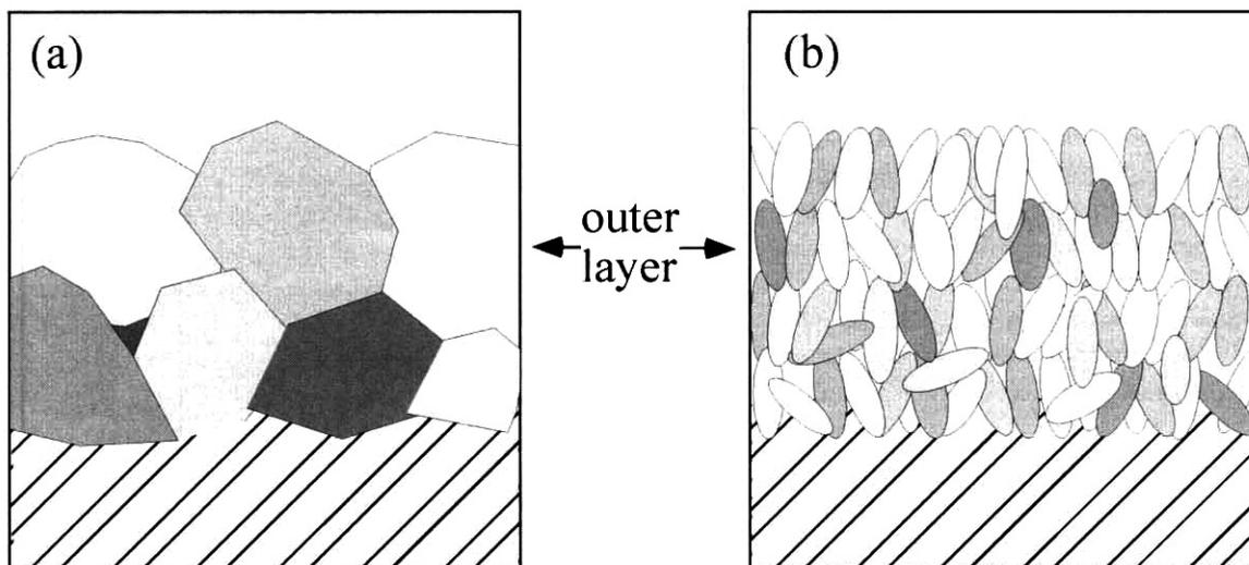
Fig. 8. Schematic representation of the structure of outer oxide layer formed on (a) Fe-19Cr, (b) Fe-19Cr-0.2Ti alloys at 1273 K in 16.5 kPa O<sub>2</sub> bal. N<sub>2</sub> for 10.8 ks.
