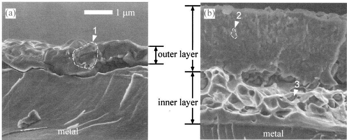
Fig. 5. SEM photographs of the oxide films formed on (a) Fe-19Cr and (b) Fe-19Cr-0.2 Ti alloys oxidized at 1273 K for 10.8 ks.
