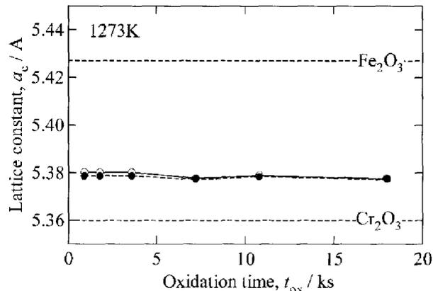
Fig. 3. Relation between oxidation time at 1273 K and lattice constants of corundum type oxides. (open marks : Fe-19Cr-0.2Ti alloy, filled marks : Fe-19Cr alloy)
