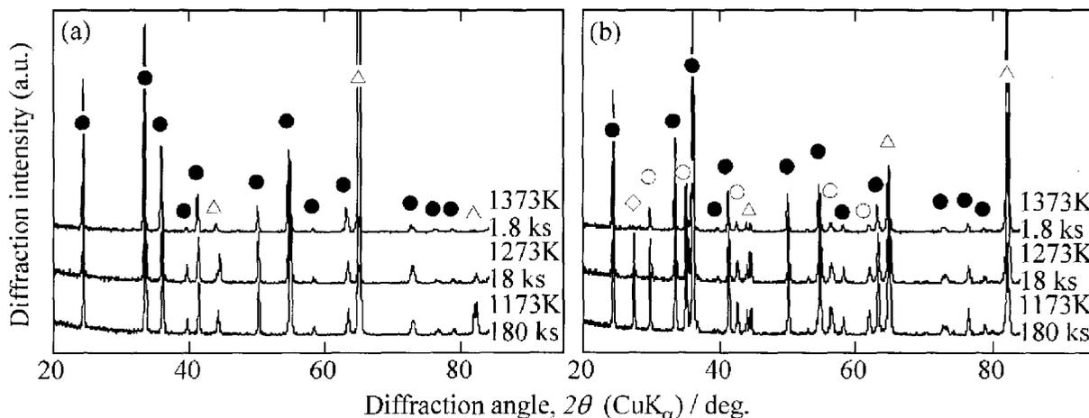
Fig. 2. XRD patterns of (a) Fe-19Cr and (b) Fe-19Cr-0.2Ti alloys after oxidation. (filled circle: Corundum type, open circle: Spinel type, triangle: substrate, diamond: Rutile)
