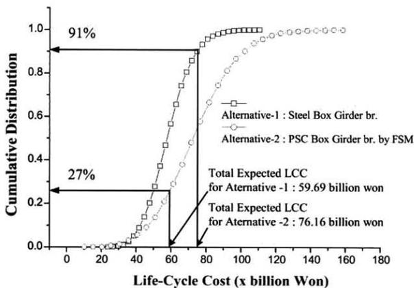
Fig. 3. Cumulative Distributions of LCC of the Two Alternatives
