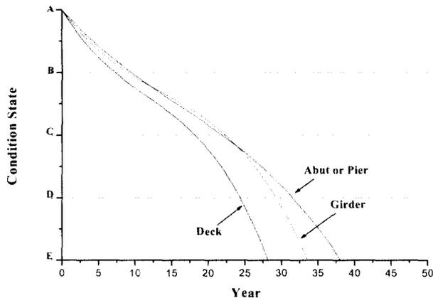
Fig. 6. CS Deterioration Curve for Deck, Main Girder and Substructure
