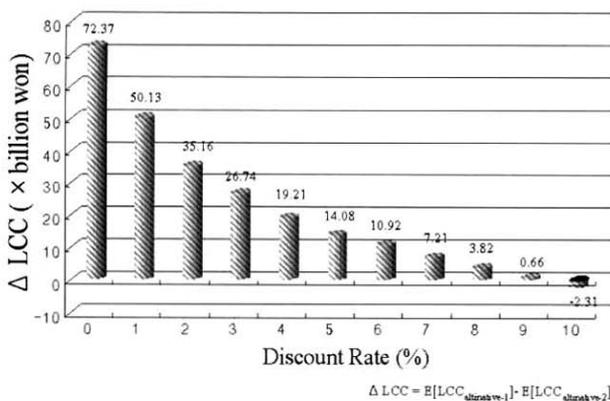
Fig. 4. Differences of Expected LCC of Two Alternatives according to Variation of Discount Rate
