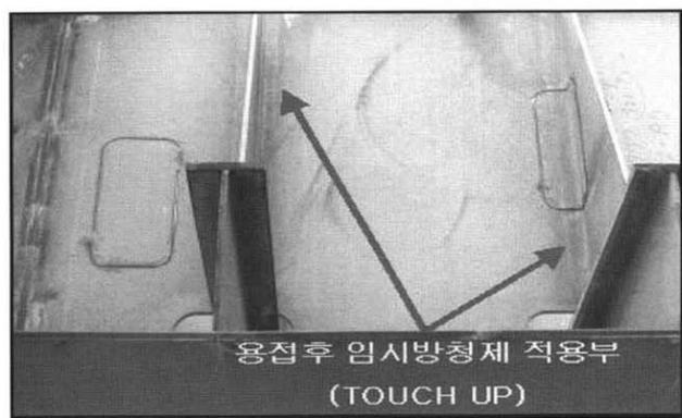
Fig. 2. Typical surface contaminations on the PCP coated blocks right after fabrication
