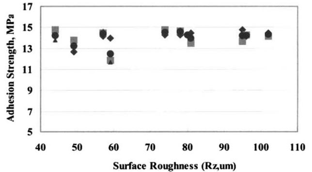
Fig. 10. Coating's adhesion strength with variation of surface roughness
