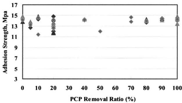
Fig. 9. Coating's adhesion strength with variation of PCP removal ratio
