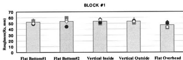
Fig. 3. Surface roughness distribution of the PCP coated blocks right after fabrication
