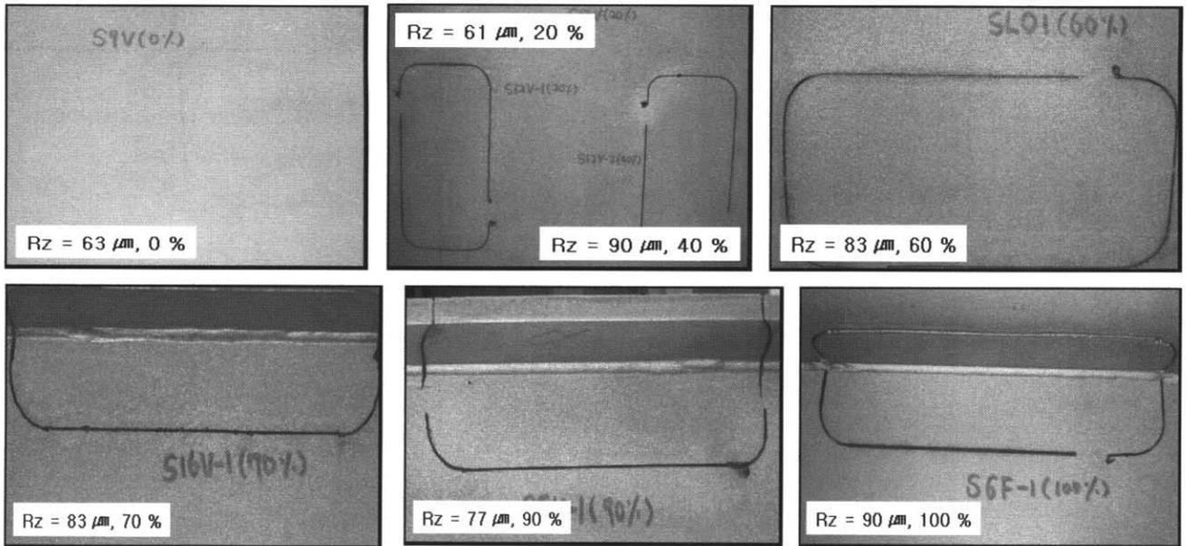
Fig. 6. Typical surface condition of the PCP coated blocks right after sweep blasting
