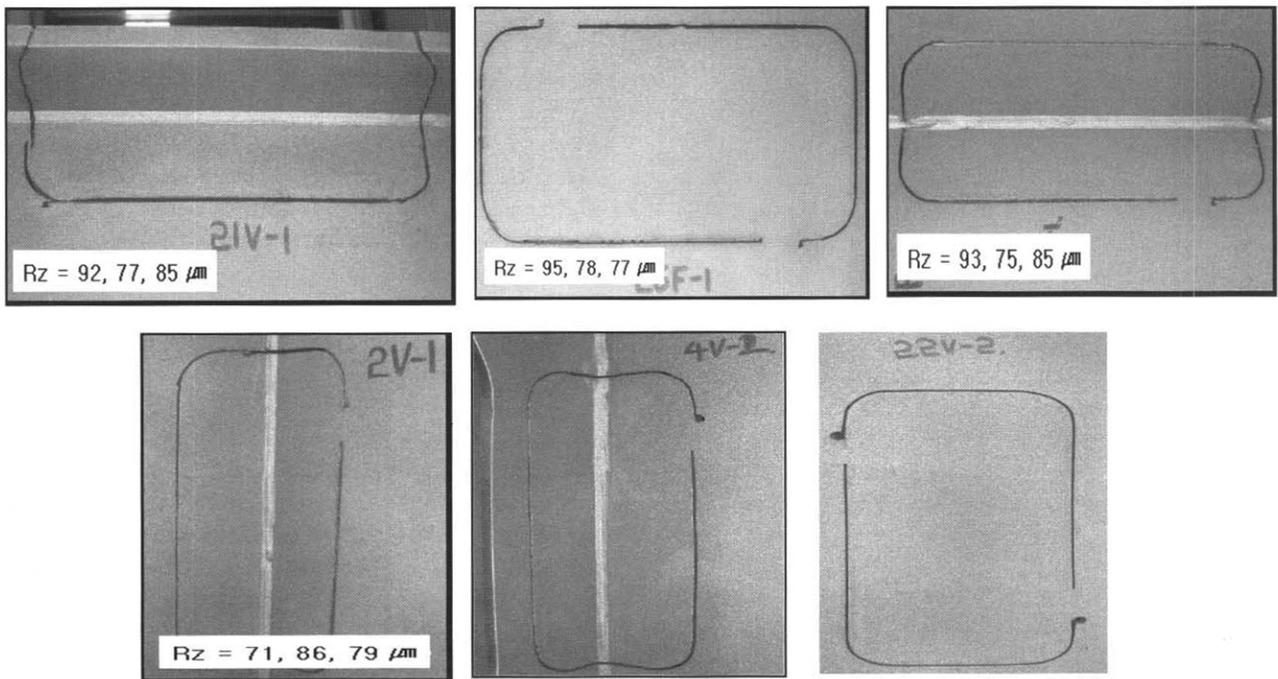
Fig. 5. Typical surface condition of the PCP coated blocks right after full blasting
