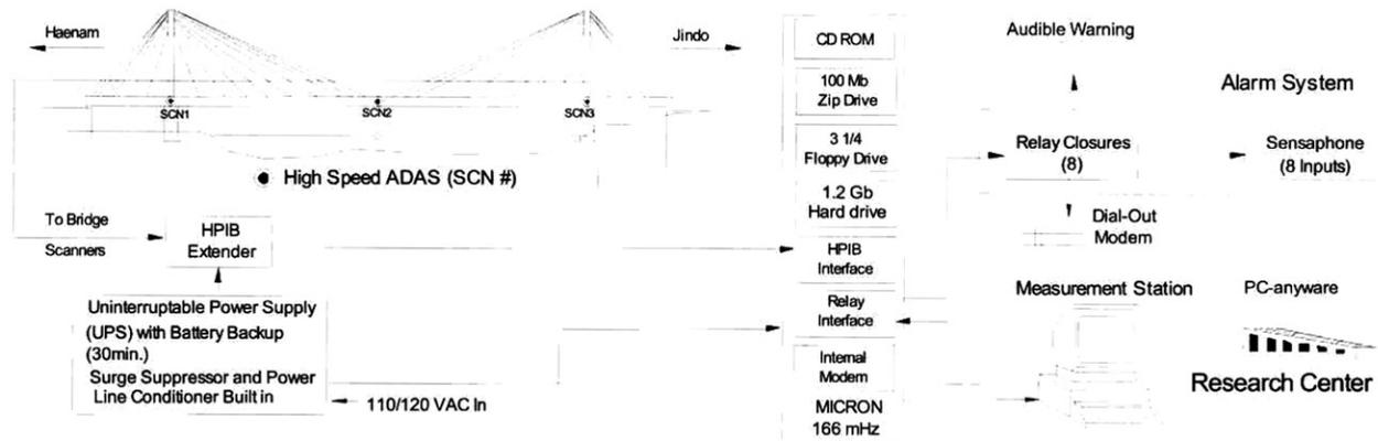
Fig. 2. Conceptual diagram of the health monitoring system installed in the Jindo bridge
