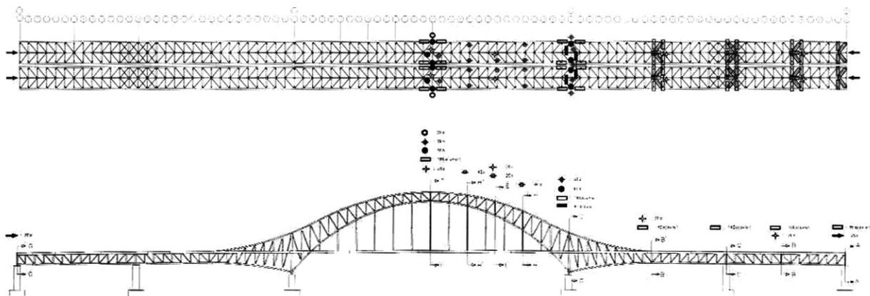
Fig. 5. Location of sensors in the Banghwa bridge
