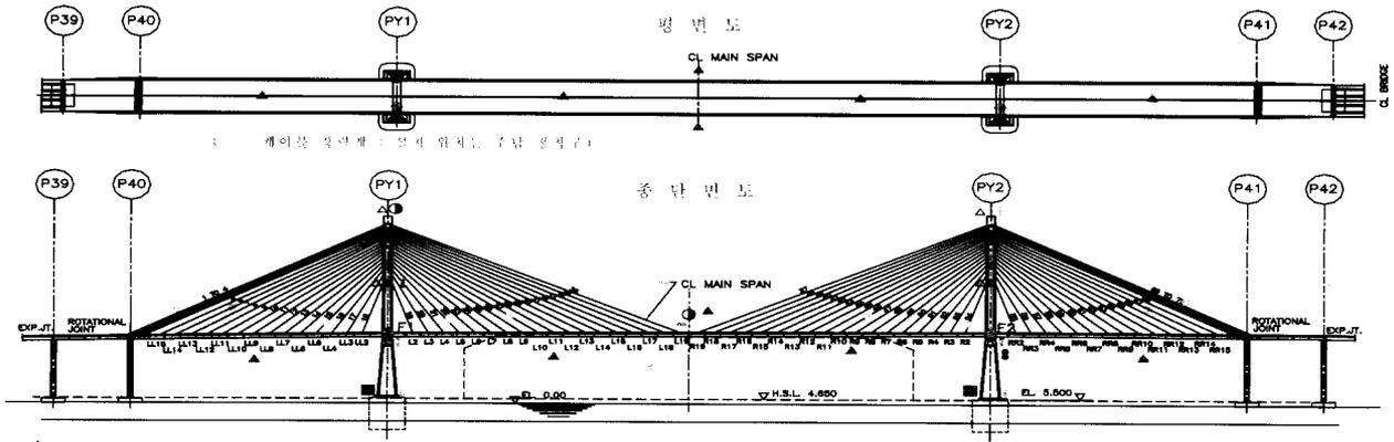
Fig. 3. Location of sensors in the Seohae bridge
