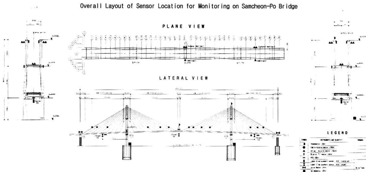
Fig. 7. Location of sensors in the Samcheonpo bridge
