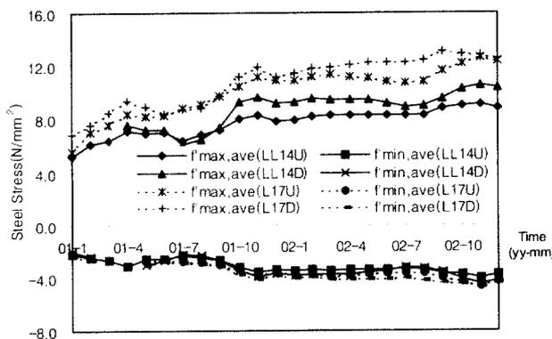
Fig. 8. Monthly variation of stress range in the lower stiffening girder flange of the Seohae bridge
