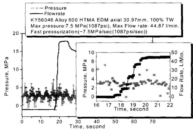
Fig. 7. Burst behavior of the through wall defect in a fast pressurization
