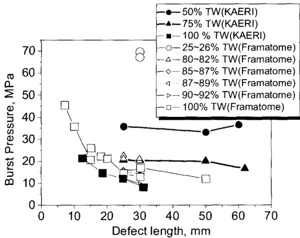
Fig. 4. Effect of the defect length on the burst pressure
