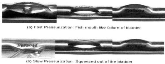
Fig. 8. Failure morphologies of the through wall defects at a different pressurization mode.
