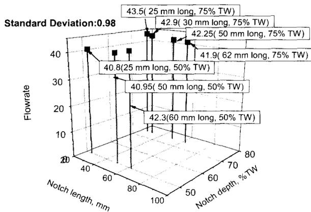
Fig. 5. Relationship among the length, depth and flow rate of the part through wall defects
