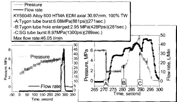
Fig. 6. Burst behavior of a through wall defect tube in a slow pressurization
