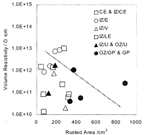
Fig. 9. Relationship between rusted area and volume resistivity.
