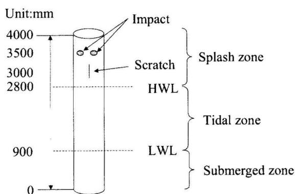
**Fig. 1.** Schematic illustration of exposed samples
