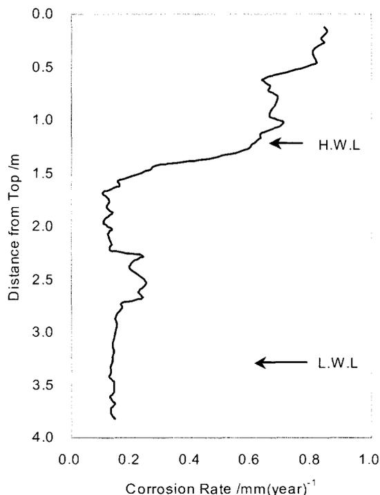
Fig. 2. Corrosion rate of bare steel pipe
