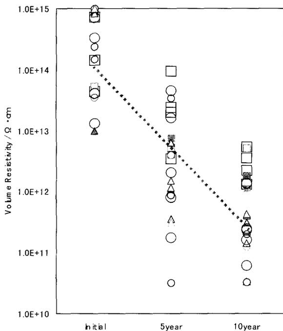
Fig. 8. Change in volume resistivity during exposure period.
