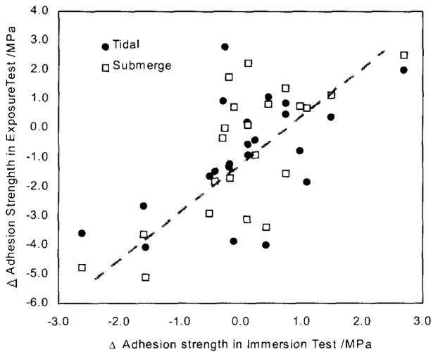
Fig. 7. Relationship in Adhesion strength between exposure and rotating immersion test
