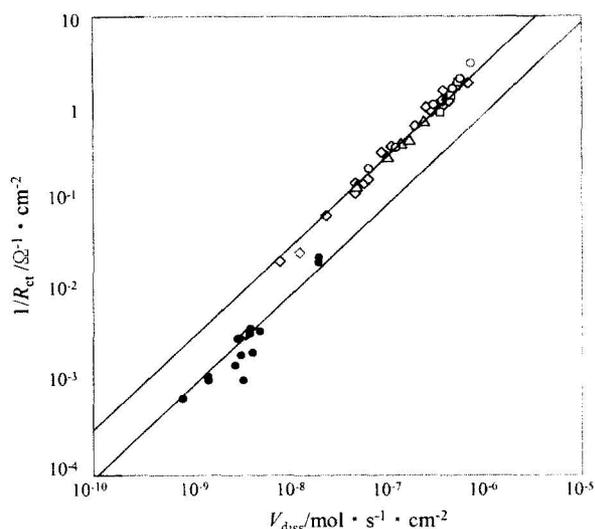
**Fig. 4.** Relation between  $R_{ct}$  and dissolution rate.
