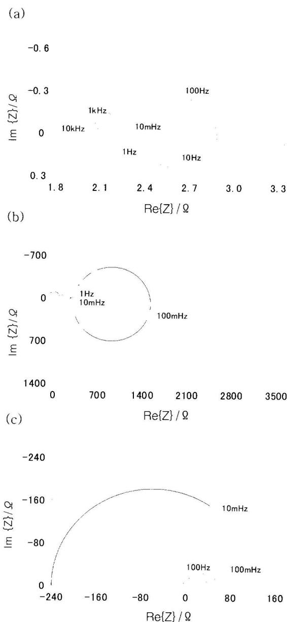
**Fig. 3.** (a) Electrochemical impedance of iron at -0.2 V vs. SSE in sulfuric acid solution (pH 1) containing  $0.03 \text{ mol/dm}^3$  NaI. (b) Electrochemical impedance of nickel at 1.3 V in sulfuric acid solution (pH 1). (c) Electrochemical impedance of nickel at 1.5 V in sulfuric acid solution (pH 1).
