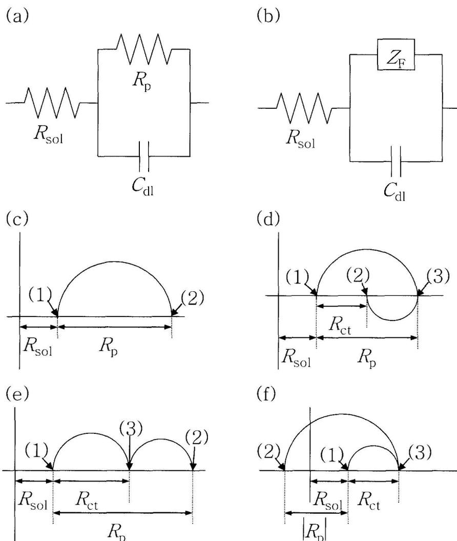
**Fig. 1.** Equivalent circuits and impedances.
