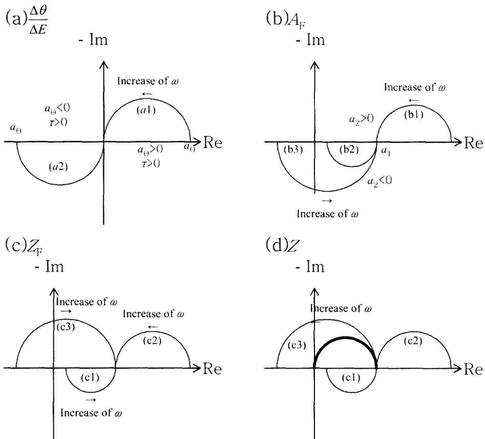
Fig. 2. Scheme of various parameters in the frequency domain: (a)  $\Delta\theta/\Delta E$ , (b) Admittance  $A_F$ , (c) Faraday impedance  $Z_F$ , (d) Impedance  $Z$ .
