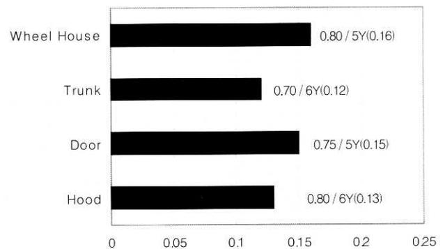
Fig. 3. Analysis results of average corrosion environment severity about field car parts (GA 60/60 applied)
