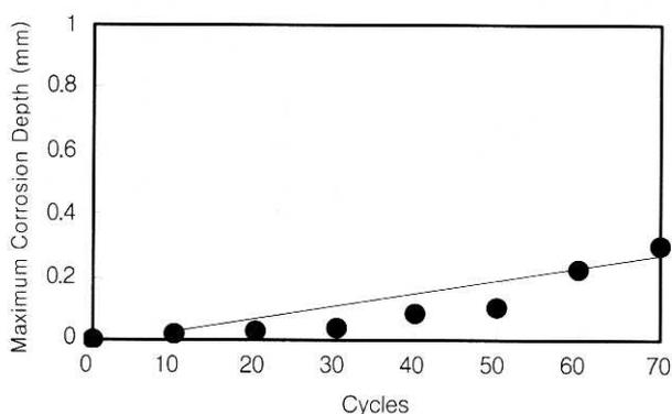
Fig. 7. Corrosion aspect at GA60/60 layer panel.(CCT (a))
