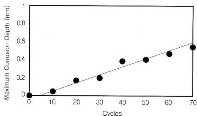
Fig. 8. Corrosion aspect at GA60/60 layer panel.(CCT (b))
