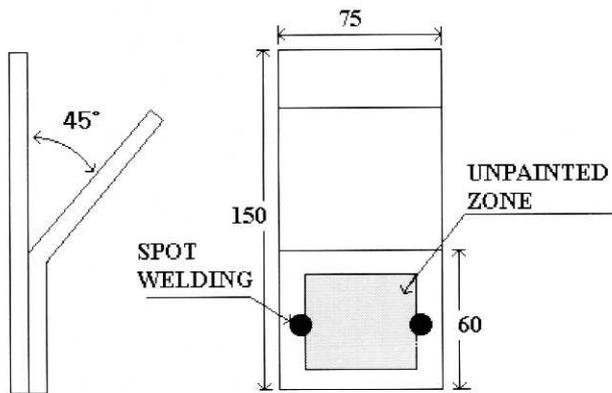
Fig. 1. Lapped Panel Specimen (unit : mm)
