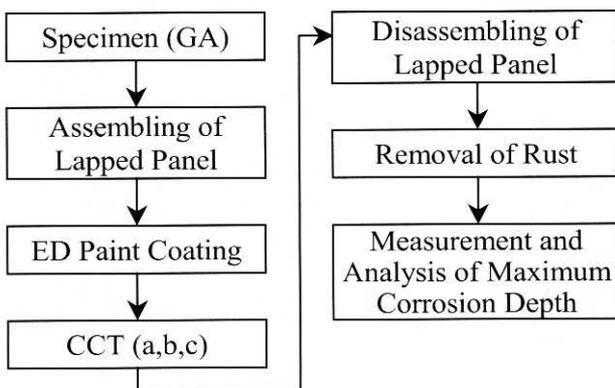
Fig. 2. Experimental Procedure
