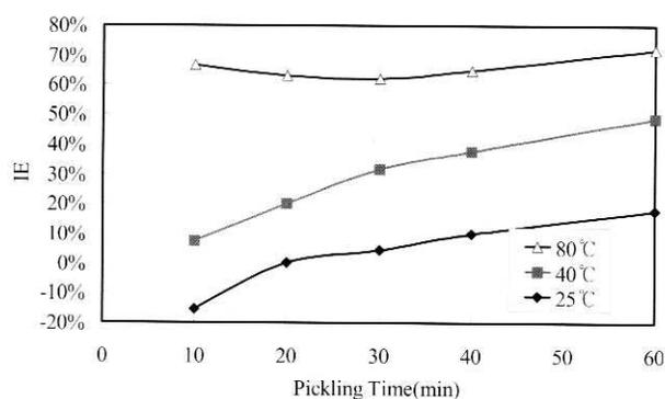
Fig. 5. The inhibition efficiency of mild steel in 12% HCl containing inhibitor B at 25°C, 40°C, and 80°C.
