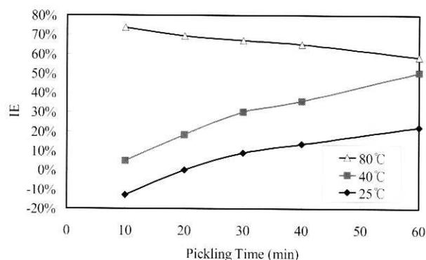
Fig. 4. The inhibition efficiency of mild steel in 12% HCl containing inhibitor A at 25°C, 40°C, and 80°C.
