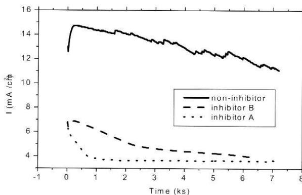
Fig. 7. Variation of current of mild steel in 12% HCl solution with/without inhibitor.
