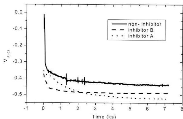
Fig. 6. Variation of potential of mild steel in 12% HCl solution with/without inhibitor.
