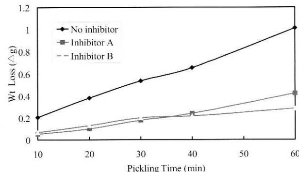
Fig. 3. Variation of weight loss with pickling time in 12% HCl solution at  $80^\circ\text{C}$ .
