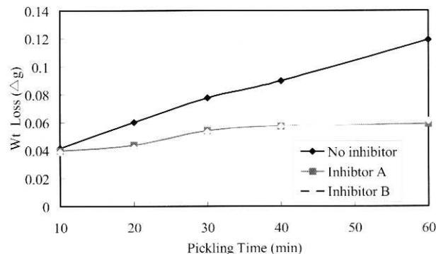
Fig. 2. Variation of weight loss with pickling time in 12% HCl solution at  $40^\circ\text{C}$ .
