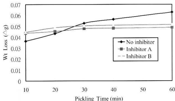
Fig. 1. Variation of weight loss with pickling time in 12% HCl solution at  $25^\circ\text{C}$ .
