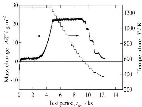
Fig. 3. Relation between mass change and temperature of SUS304 stainless steel during the test. Oxidation condition is the same as that described in Fig. 1
