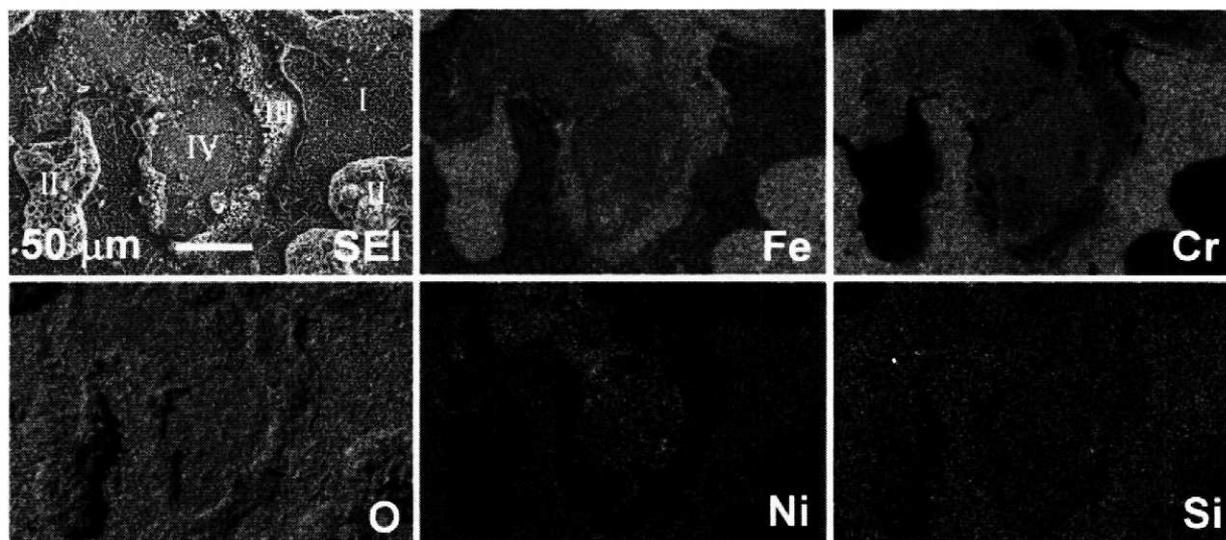
Fig. 5. Surface appearance and secondary X ray images of SUS304 stainless steel oxidized at 1273 K for 3.6 ks, and then cooled stepwise to room temperature (Run3 in table 3).
