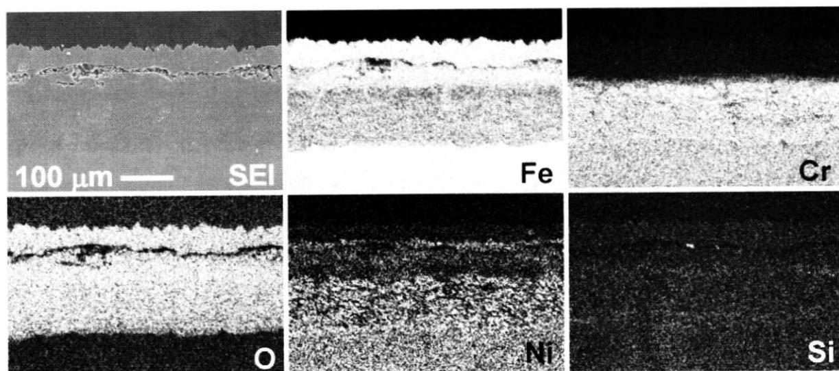
Fig. 9. Secondary electron image and X ray images of the cross section for SUS304 stainless steel after a cyclic oxidation test shown in Fig. 7.
