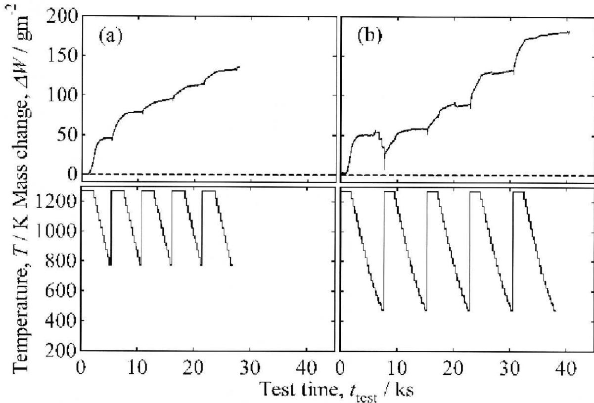
Fig. 7. Changes in mass and the temperature of SUS304 stainless steel during a cyclic oxidation test in 16.7 kPa O<sub>2</sub> - 20.3 kPa H<sub>2</sub>O - balanced N<sub>2</sub> atmosphere. The isothermal oxidation at 1273 K continues 3.6 ks and the cycle repeated while the temperature of the specimen decreased at (a) 773 K and (b) 473 K.
