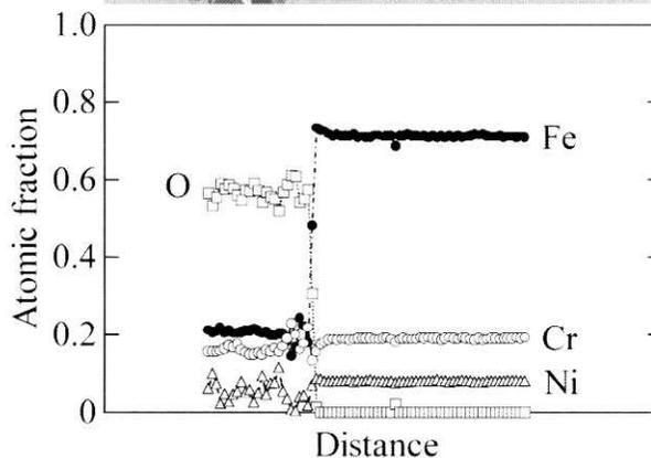
Fig. 4. Cross section and a result of EPMA analysis. The annotation in the picture is the same as that described in Fig. 2.
