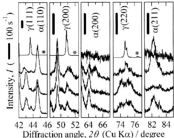
**Fig. 6.** The X-ray diffraction patterns of SUS304 stainless steels. Curve (1) was taken before oxidation test and (2), (3), and (4) were taken after the test and correspond to Run 2, 3, and 7 in table 3. Curves with a mark (\*) are compressed 1/100 with Y-axis.
