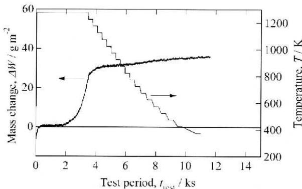
**Fig. 1.** Relation between mass change of SUS430 stainless steel,  $\Delta W$ , and test period,  $t_{test}$ , during high temperature oxidation test in 16.7 kPa  $O_2$  - 20.3 kPa  $H_2O$ - balanced  $N_2$ . Change in the specimen temperature is also shown.
