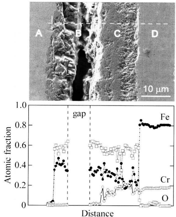
**Fig. 2.** A cross section and result of EPMA analysis of SUS430 stainless steel oxidized at  $T_{ox} = 1273 \text{ K}$  for  $t_{heat} = 3.48$  ks, and then cooled stepwise to room temperature (Run 7 in Table 2). Broken line in the picture is the analyzed portion, region A is Ni plating for observation, B an outer oxide scale, C an inner scale, and D substrate alloy.
