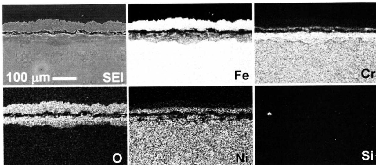
Fig. 8. Secondary electron image and X ray images of the cross section for SUS304 stainless steel after a cyclic oxidation test shown in Fig. 7.
