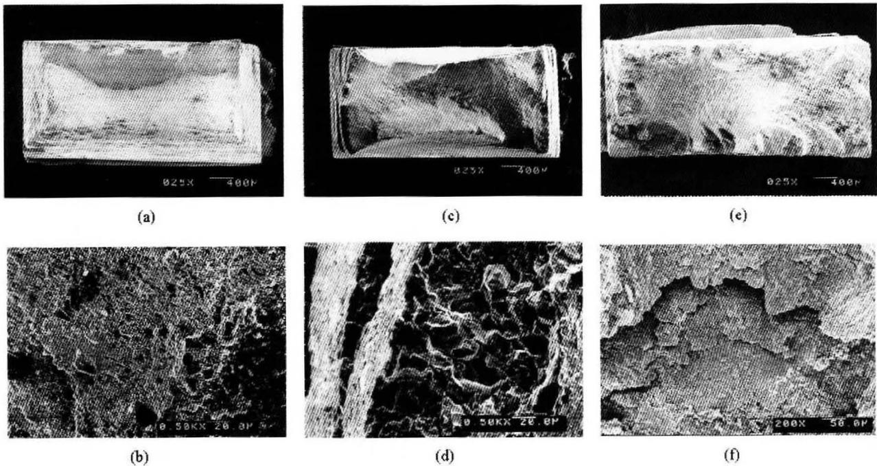
Fig. 5. Fracture surfaces failure in SSRT test at  $150^\circ\text{C}$ ; (a) Deaerated water - top view, (b) Deaerated water - enlargement showing ductile rupture, (c) Intermediated - top view, (d) Intermediated - enlargement showing IGSCC, (e) Aerated water - top view, (f) Aerated water - enlargement showing IGSCC.
