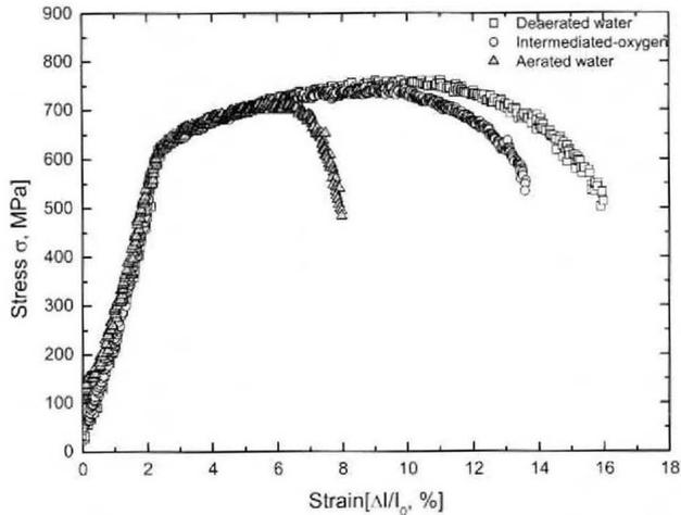
Fig. 3. Stress strain curves produced form data recorded during SSRT test results in varied environments with the strain rate of  $10^{-7} \text{ s}^{-1}$  at  $150^\circ\text{C}$ .
