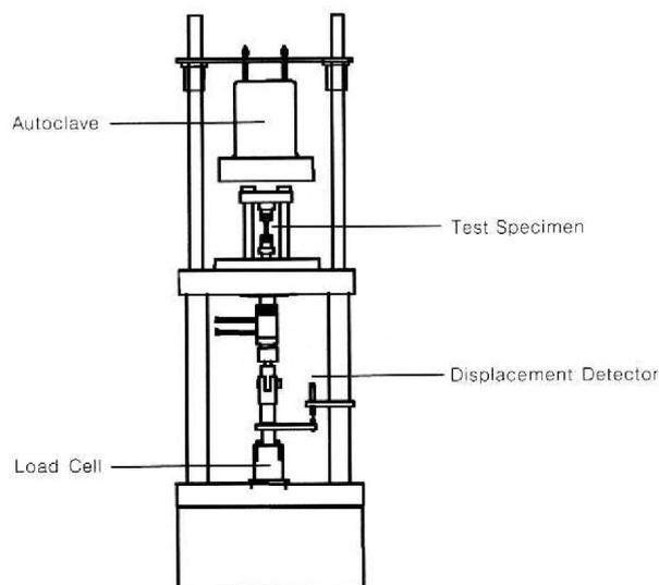
**Fig. 2.** Schematic drawing of the slow strain rate tester.
