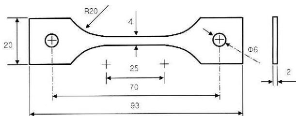
**Fig. 1.** Geometry of SSRT test specimen (unit: mm).
