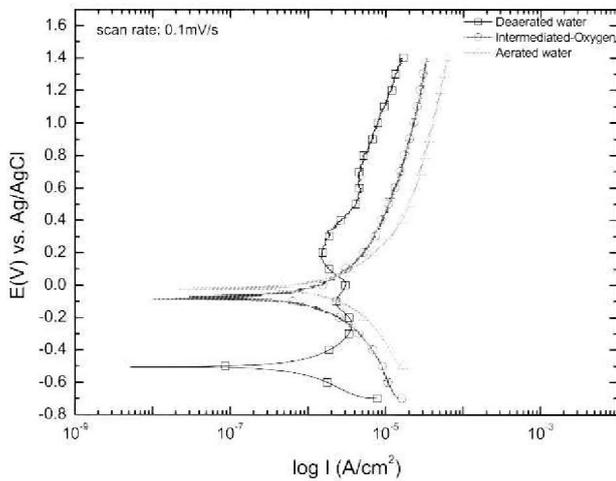
Fig. 7. Polarization curves of 3.5NiCrMoV steel in varied environments at  $150^\circ\text{C}$ : scan rate- $0.1\text{mV/s}$ .
