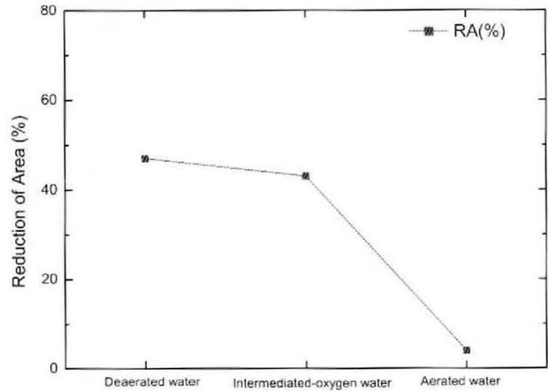
Fig. 4. Reduction area value of SSRT test results in varied environments with the strain rate of  $10^{-7} \text{ s}^{-1}$  at  $150^\circ\text{C}$ .
