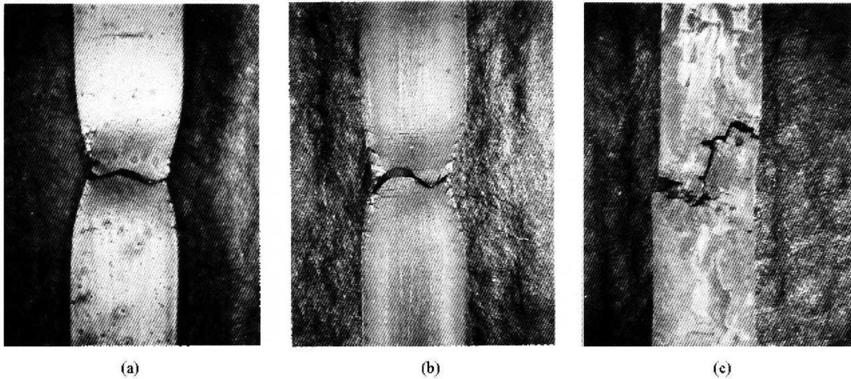
Fig. 6. Fracture morphologies tested in varied environments with the strain rate of  $10^{-7} \text{ s}^{-1}$  at  $150^\circ\text{C}$ ; (a) Deaerated water, (b) Intermediate, (c) Aerated water.
