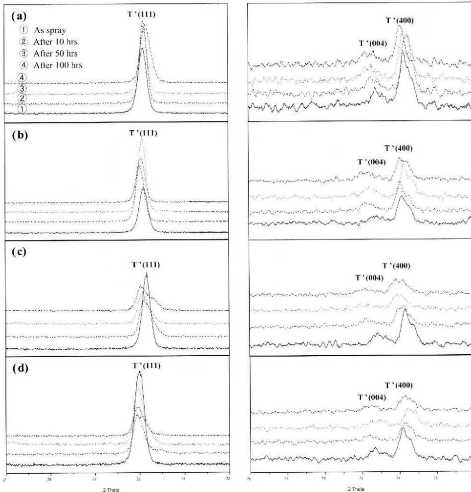
Fig. 4. The change in X-ray diffraction patterns of ZrO<sub>2</sub> coating layers having four different types of grading with variation of oxidation time. (a) TBC(T) (b) symmetry four-graded layer (F1) (c) symmetry four-graded layer (F2) (d) ceramic rich four-graded layer (F3)
