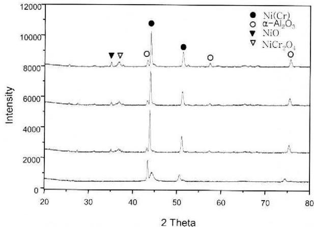
Fig. 7. The change of X-ray diffraction patterns of NiCrAlY bond layers with variation of oxidation time.
