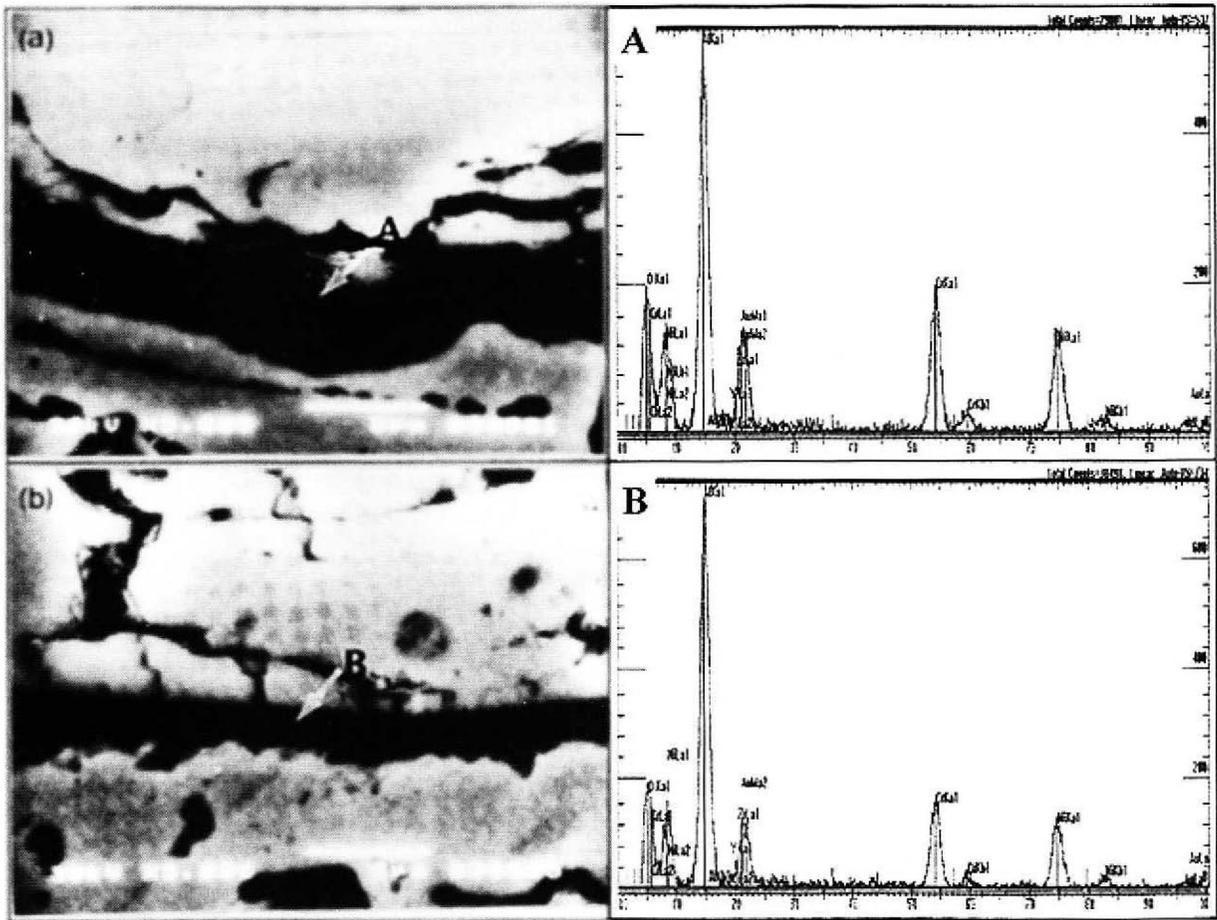
Fig. 6. SEM micrographs and EDS analysis of ZrO<sub>2</sub> coating layers having four different types of grading with variation of oxidation time. (a) TBC(T), after 100 hours (b) FGC(F2), after 50 hours
