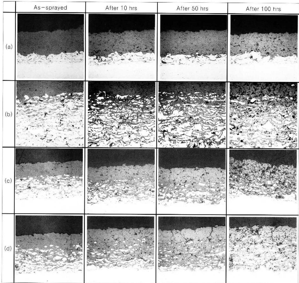
Fig. 1. Microstructural change in four ZrO<sub>2</sub> coating layers having four different types of grading with variation of oxidation time. (a) TBC(T) (b) symmetry four-graded layer (F1) (c) symmetry four-graded layer(F2) (d) ceramic rich four-graded layer(F3)
