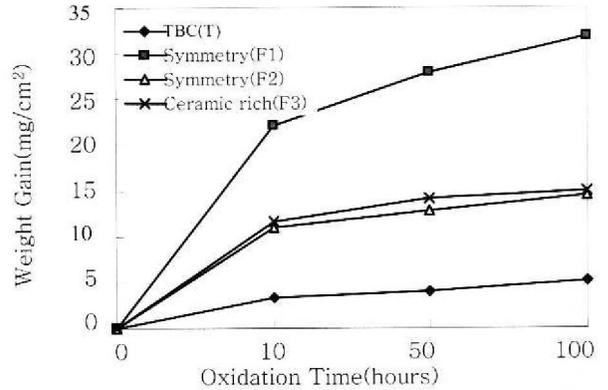
Fig. 5. Weight change of ZrO<sub>2</sub> coating layers having four different types of grading with variation of oxidation time.
