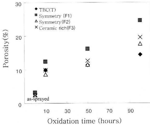
Fig. 3. Change in porosity in TBC and FGC samples (T, F1, F2, F3) with variation of oxidation time.
