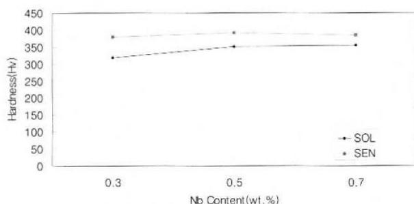
Fig. 3. Hardness of the solutionized and sensitized stainless steels as function of Nb content.
