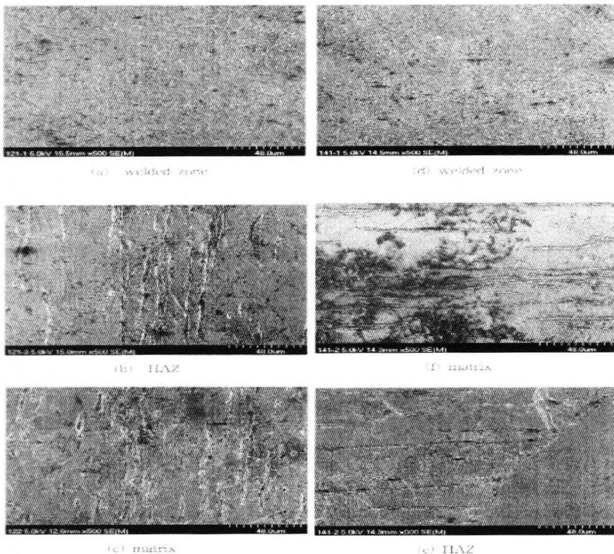
Fig. 13. SEM micrographs showing the intergranular corrosion of welded stainless steels containing 0.3 wt%(a,b,c) and 0.7 wt%(d,e,f) Nb after EPR test in 0.1M H<sub>2</sub>SO<sub>4</sub> + 0.01M KSCN solution at 25°C.
