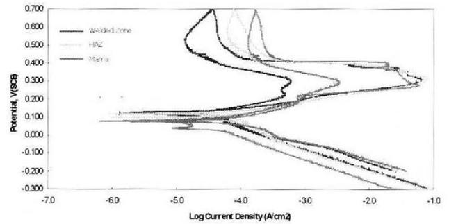
Fig. 10. EPR curves for the welded zone, HAZ, and the matrix of stainless steels containing 0.3 wt% Nb in 0.1M  $H_2SO_4$  + 0.01M KSCN solution at 25°C.
