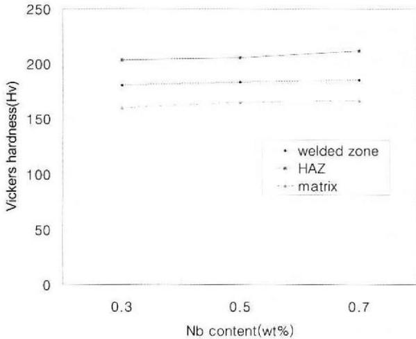
Fig. 9. Micro-vickers hardness of welded zone, HAZ, and matrix for stainless steels as function of Nb content.
