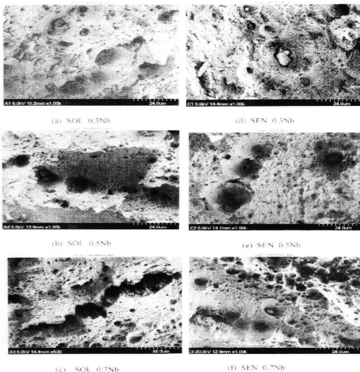
Fig. 5. SEM fractographs of the solutionized(a,b,c) and sensitized (d,e,f) stainless steels containing Nb after tensile test.
