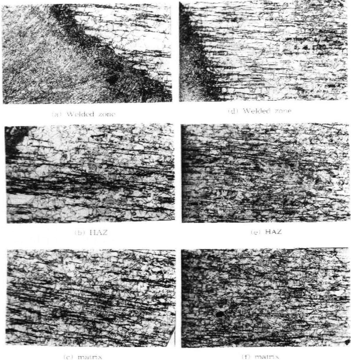
Fig. 8. Optical micrographs of welded stainless steels containing 0.3 wt%(a, b, c) and 0.5 wt%(d, e, f) Nb after etching in 10% oxalic acid.
