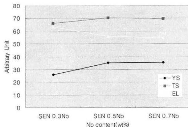
Fig. 4. Results of tensile test of the sensitized stainless steels.
