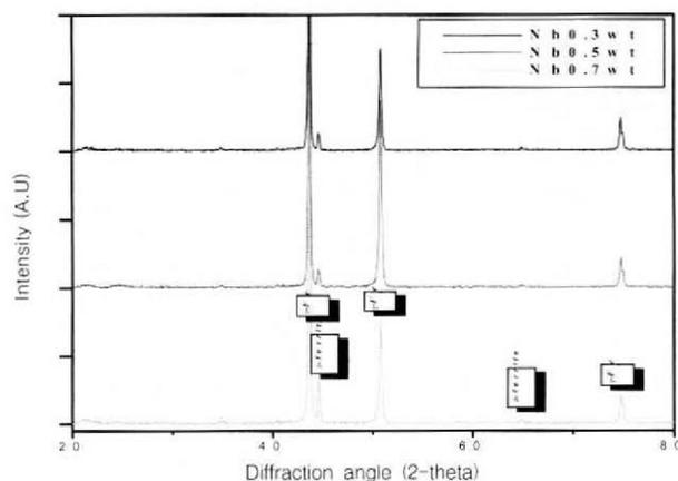
Fig. 2. X-ray diffraction patterns of the solutionized stainless steels containing Nb.
