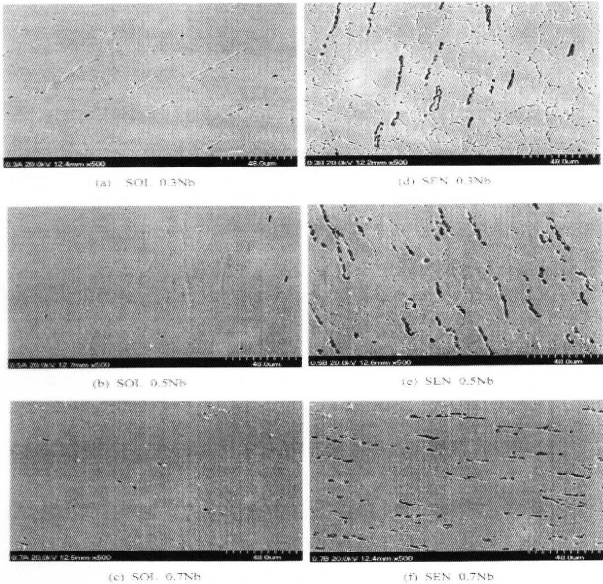
**Fig. 6.** SEM micrographs showing intergranular corrosion of the solutionized(a,b,c) and sensitized (d,e,f) stainless steels containing Nb after corrosion test in oxalic acid.
