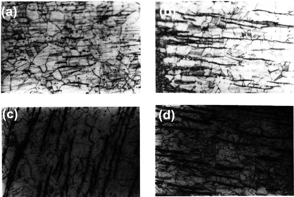
Fig. 1. Optical micrographs of SOL0.3Nb(a), SOL0.7Nb(b), SEN0.3Nb(c) SEN0.7Nb(d) after etching in 10% oxalic acid.
