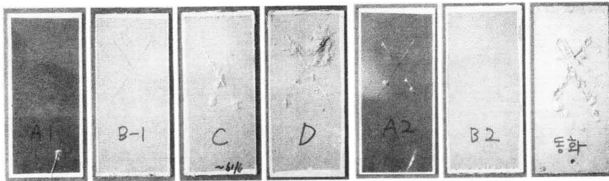
Fig. 5. Test results of salt spray for several coating finished plates
