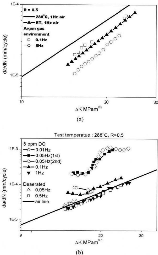
**Fig. 1.** Fatigue crack growth rate of SA 508 Cl.3 (a) in argon and air environment, (b) in water environment
