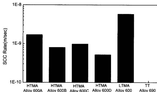
**Fig. 2. SCC Rate of Steam Generator Materials in 10% NaOH at 315°C**
