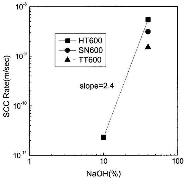
Fig. 3. NaOH concentration dependency of SCC rate at an initial stress of 340MPa and at 315°C and at 200mV above corrosion potential.
