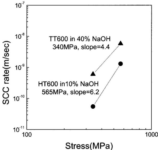
Fig. 4. Stress dependency of SCC rate.
