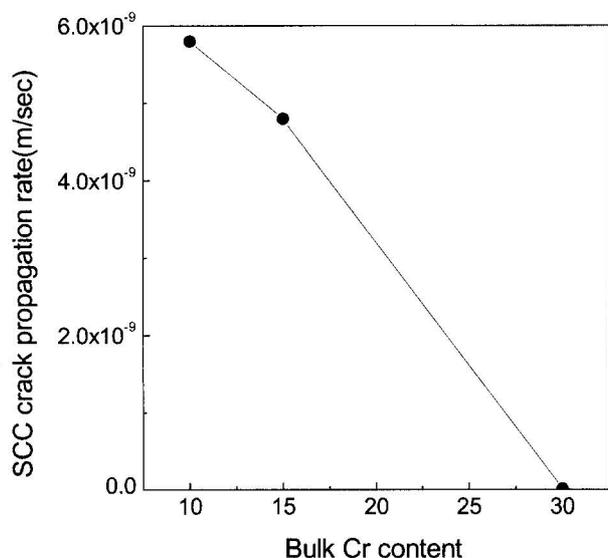
Fig. 1. Effect of bulk Cr content in Ni- $\chi$ Cr-10Fe alloy on SCC crack propagation rate.
