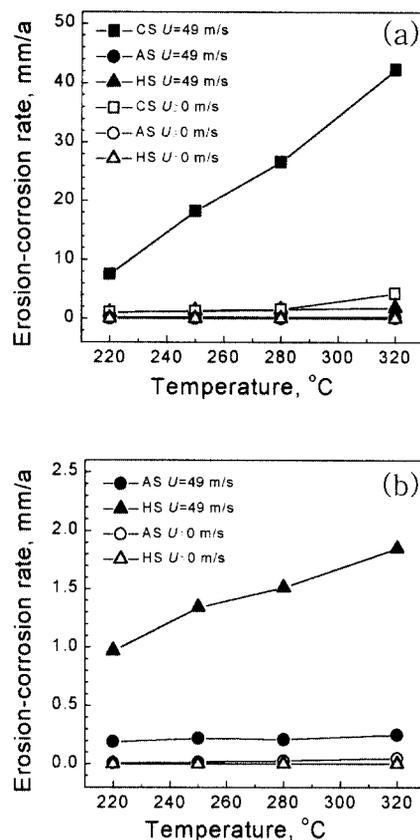
Fig. 3. NAEC rate at high temperature of (a) CS, AS and HS, (b) AS and HS
