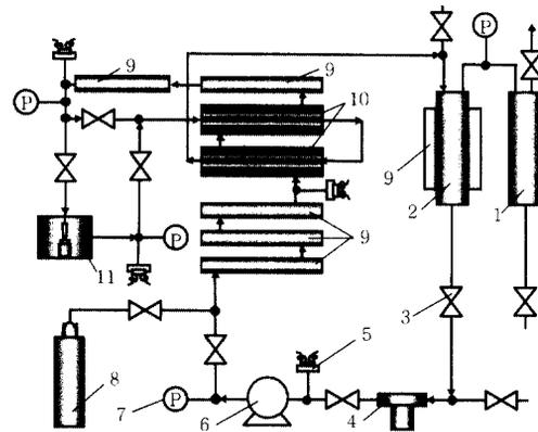
1-releaser, 2-oil reservoir, 3-valve 4-filter, 5- thermocouple, 6-pump, 7- pressure gauge, 8- $N_2$  container, 9-heater, 10-heat exchangers, 11-jet impingement chamber
