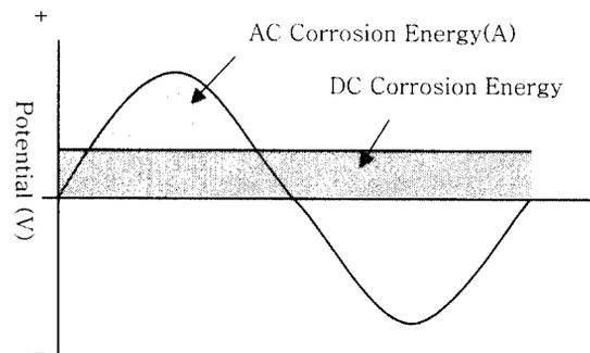
Fig. 5. AC & DC potential used corrosion energy
