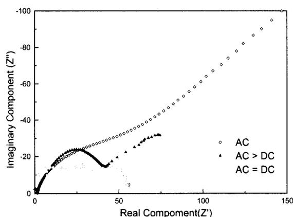
Fig. 7. E.I.S. test result of SS 40 in sea water
