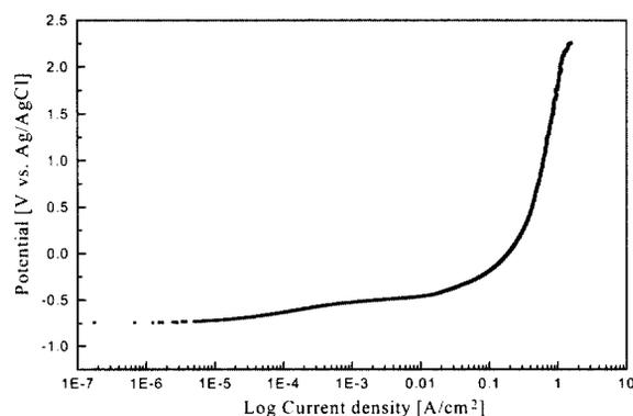
Fig. 6. Polarization curve of the SS 40 in sea water
