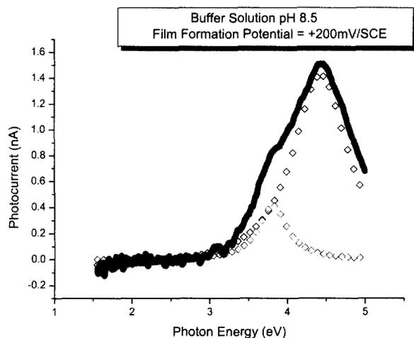
**Fig. 3.** Photocurrent spectra for the passive film formed on Fe-18Ni-8Ni-4Mo at +200 mV<sub>SCE</sub> in deaerated pH 8.5 buffer solution, and its resolution into its component spectrum.
