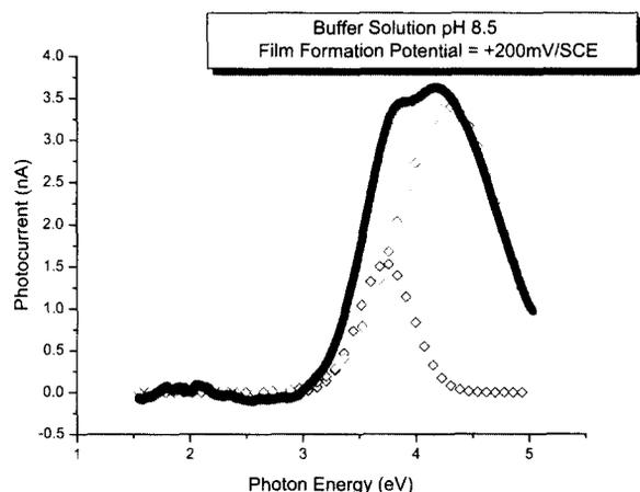
**Fig. 2.** Photocurrent spectra for the passive film formed on Fe-18Ni-8Cr at +200 mV/SCE in deaerated pH 8.5 buffer solution, and its resolution into its component spectrum.
