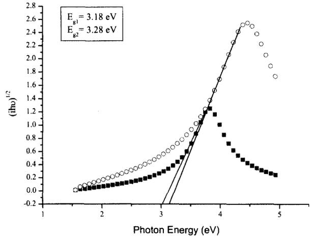
**Fig. 6.** Determination of the optical band gap energy for the passive film formed on Fe-18Ni-8Cr-4Mo SS at 200 mV<sub>SCE</sub> in pH 8.5 buffer solution.
