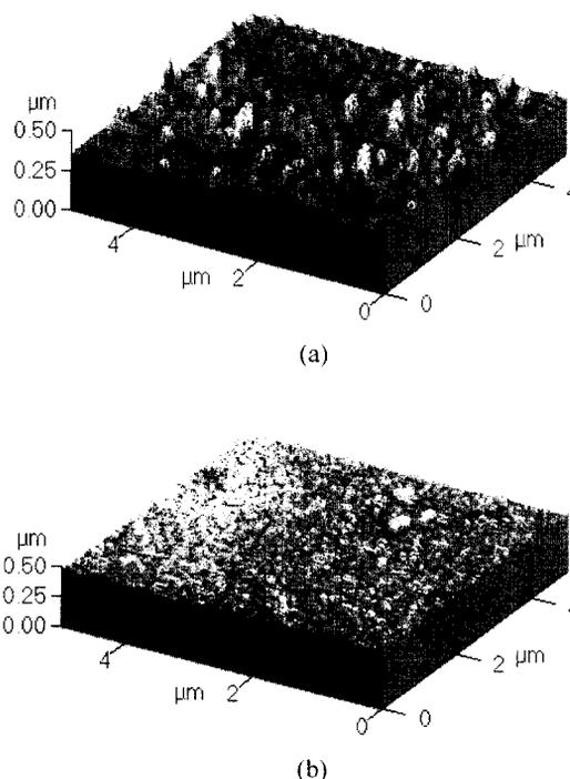
**Fig. 9.** Three-dimensional AFM topography for the passive films formed on 18Cr-8Ni (a) and 18Cr-8Ni-4Mo (b) alloys. The passive films were grown for 24 hr at 200mV<sub>SCE</sub> in pH 8.5 buffer solution.
