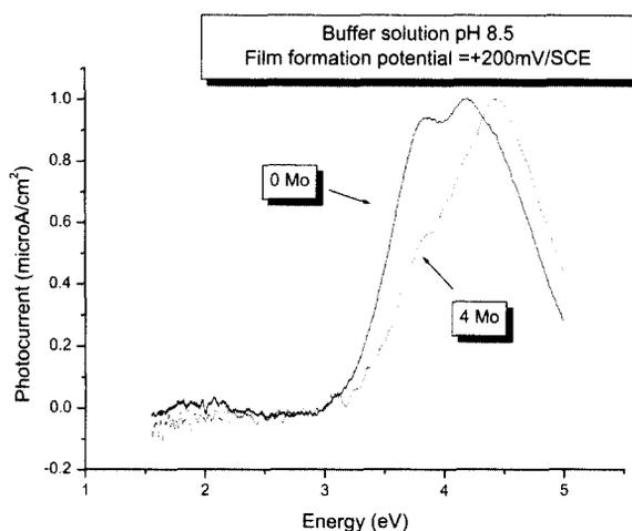
**Fig. 4.** Normalized photocurrent spectra for the passive films on Fe-18Cr-8Ni and Fe-18Cr-8Ni-4Mo polarized for 24 hrs. at +200mV<sub>SCE</sub> in pH 8.5 buffer solution.
