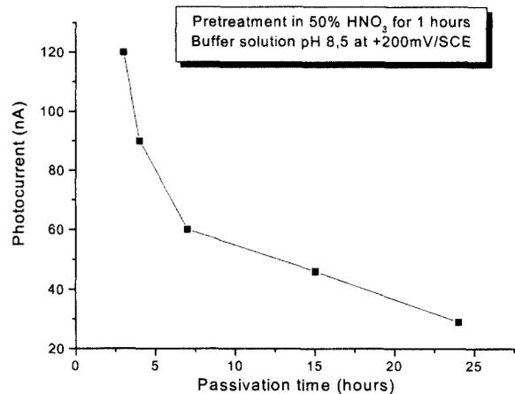
**Fig. 7.** Decrease in the peak photocurrent with polarization time at 200 mV<sub>SCE</sub> for the passive film formed on pre-acid treated 18Cr-8Ni SS.
