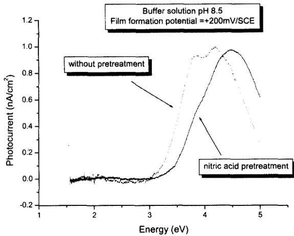
**Fig. 5.** Effects of pre-acid treatment on the photocurrent spectrum for the passive film on Fe-18Cr-8Ni in pH 8.5 solution; the pre-acid treatment was done by exposing the alloy to 50% HNO<sub>3</sub> solution for 1 hour.
