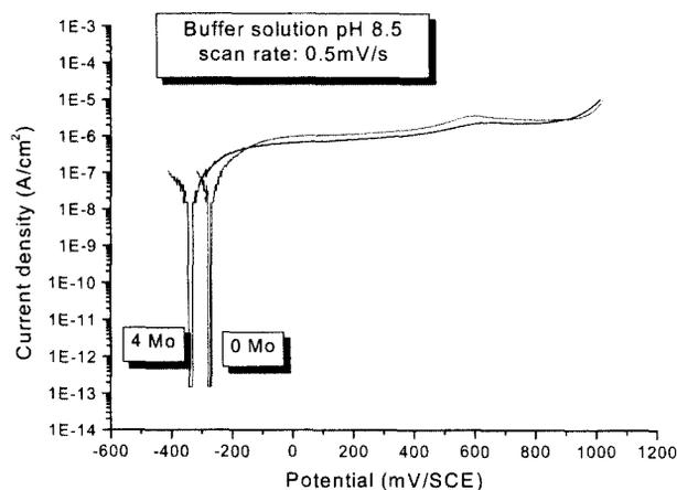
Fig. 1. Potentiodynamic polarization responses for Fe-18Cr-8Ni and Fe-18Cr-8Ni-4Mo SSs in the pH 8.5 buffer solution at 25 °C.
