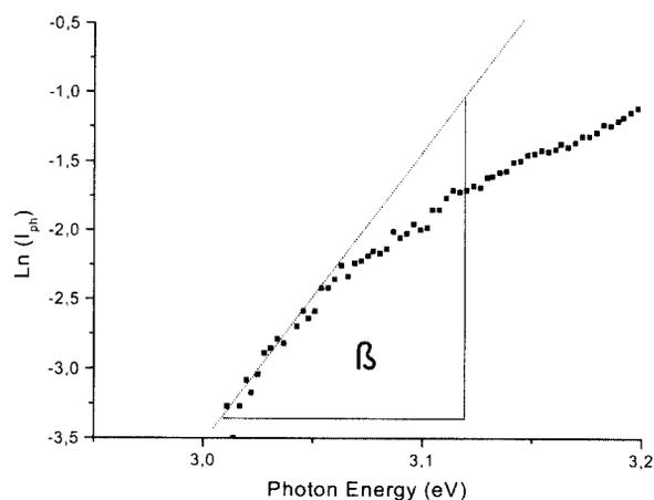
**Fig. 8.** Evaluation of the disorder energy from the plot of  $\ln(i_{ph})$  vs.  $h\nu$  for the passive films on Fe-18Cr-8Ni polarized for 24 hrs. at +200mV<sub>SCE</sub> in pH 8.5 buffer solution
