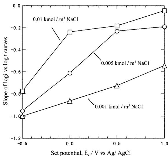
**Fig. 11.** Effect of set potential,  $E_s$ , and chloride ion concentrations on the slope of  $\log t$  vs.  $\log t$  curves.
