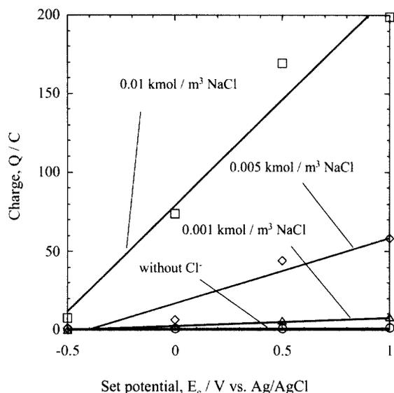
**Fig. 10.** Effect of the set potential,  $E_s$ , and chloride ion concentrations on the charge,  $Q$ .
