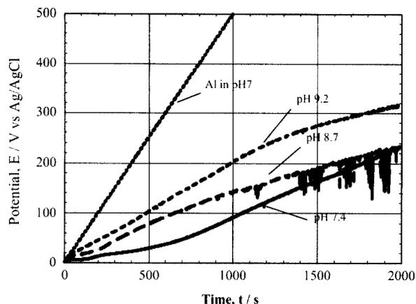
**Fig. 2.** Potential time response for Al and Zn - 55 mass % Al coated steel at  $10 \text{ A / m}^2$  in  $0.1 \text{ kmol / m}^3 \text{ Na}_2\text{B}_4\text{O}_7$  (pH = 9.2),  $0.1 \text{ kmol / m}^3 \text{ H}_3\text{BO}_3 / 0.05 \text{ kmol / m}^3 \text{ Na}_2\text{B}_4\text{O}_7$  (pH = 8.7), and  $0.5 \text{ kmol / m}^3 \text{ H}_3\text{BO}_3 / 0.05 \text{ kmol / m}^3 \text{ Na}_2\text{B}_4\text{O}_7$  (pH = 7.4) solutions.
