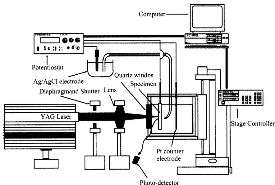
Fig. 1. Schematic diagram of laser irradiation system with electrochemical current measurement unit.
