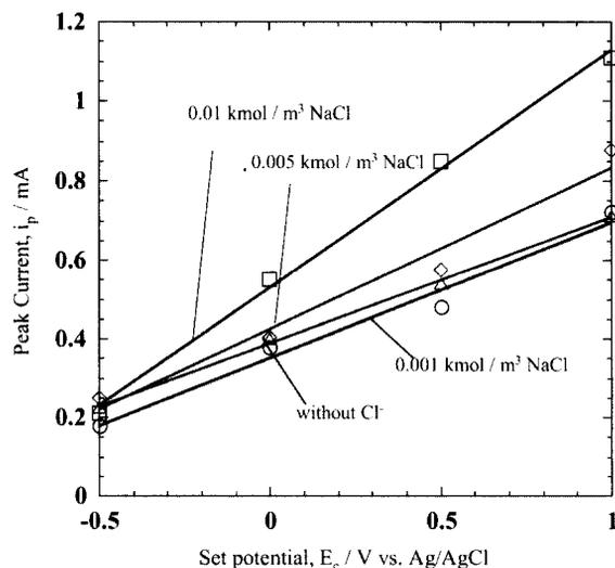
Fig. 9. Effect of the set potential,  $E_s$ , and chloride ion concentrations on the peak current,  $i_p$ .
