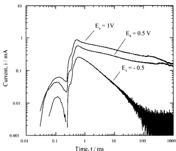
Fig. 7. Change in current with time obtained in  $0.1 \text{ kmol} / \text{m}^3 \text{ Na}_2\text{B}_4\text{O}_7$  with  $0.005 \text{ kmol} / \text{m}^3 \text{ NaCl}$  solution at  $E_s = -0.5$ ,  $0.5$  and  $1.0 \text{ V}$  after laser irradiation.
