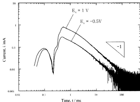
Fig. 6. Change in the current with time obtained in  $0.1 \text{ kmol} / \text{m}^3 \text{ Na}_2\text{B}_4\text{O}_7$  solution at  $E_s = -0.5$  and  $1.0 \text{ V}$  after laser irradiation.
