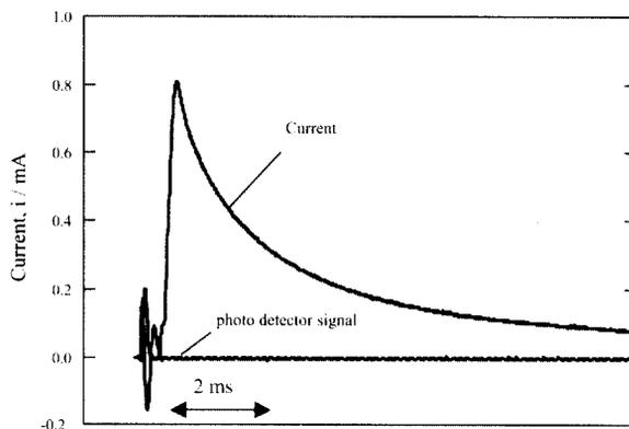
**Fig. 5.** Current transient and photo detector signal between 0 to 10 ms after laser irradiation at  $E_s = -0.5$  in  $0.1 \text{ kmol / m}^3 \text{ Na}_2\text{B}_4\text{O}_7$  solution.
