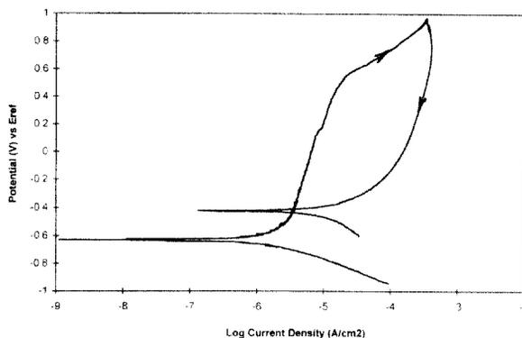
Fig. 1. Cyclic potentiodynamic curve of unprotected reinforcement submerged cyclically in 3.5% NaCl solution
