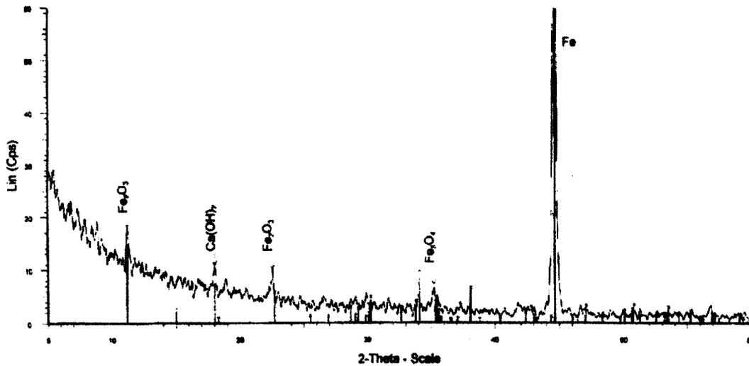
Fig. 6. X-ray diffractogram of protected-at-7 mA/m<sup>2</sup> reinforcement submerged continuously in 3.5% NaCl solution
