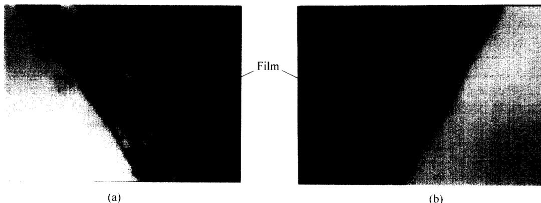
Fig. 4. Cross sections of the unprotected (a) and protected-at-13 mA/m<sup>2</sup> (b) reinforcements submerged cyclically in 3.5% NaCl solution
