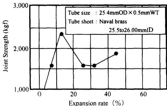
Fig. 3. Effect of expansion rate on joint strength when using a sealant between tube and tube sheet
