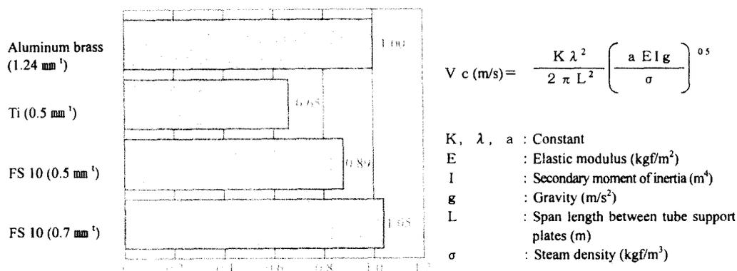
Fig. 4. Relative critical steam velocity affecting vibration resistance of commercialized condenser tubes
