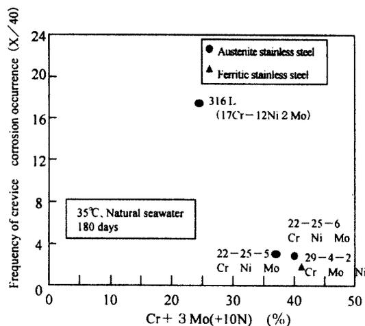
**Fig. 2. Effect of alloying elements on crevice corrosion resistance**
