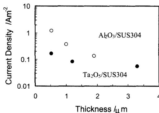
**Fig. 1.** Relationship between CPCD and oxide film thickness
