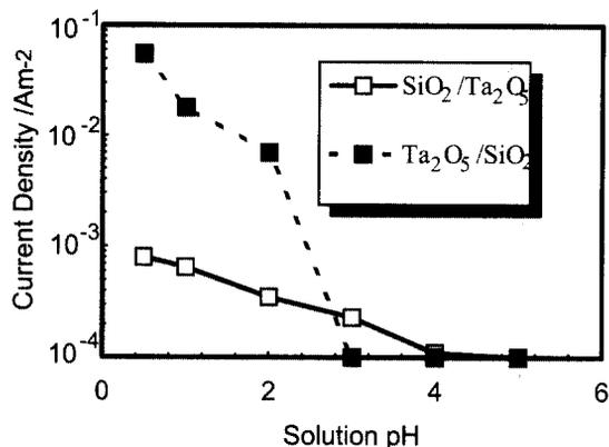
Fig. 4. Behavior of passive current in various solution pH
