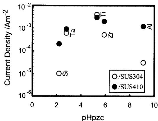
Fig. 2. Relation between passive current density and  $pH_{pzc}$  of oxide film
