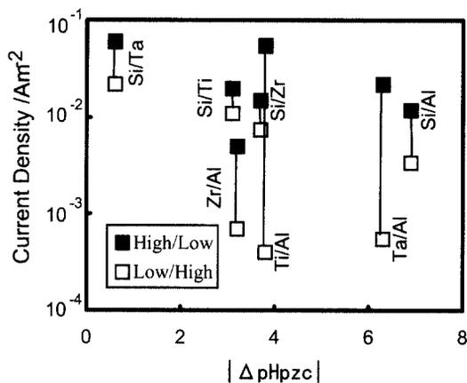
Fig. 3. Relation between passive current density and  $pH_{pzc}$  difference of dual-layered oxide film
