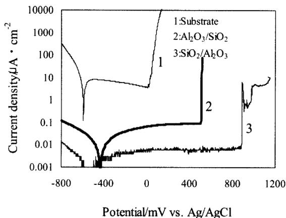
Fig. 5. Anodic polarization curves of the double-layered oxide coated steels measured in buffer solution containing  $1.0 \text{ kmol/m}^3$  NaCl of  $\text{pH}=5.4$ .
