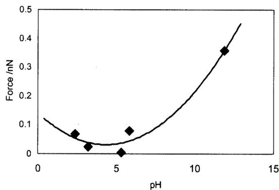
Fig. 6. Relation between repulsive force and solution pH for  $\text{TiO}_2$  oxide film
