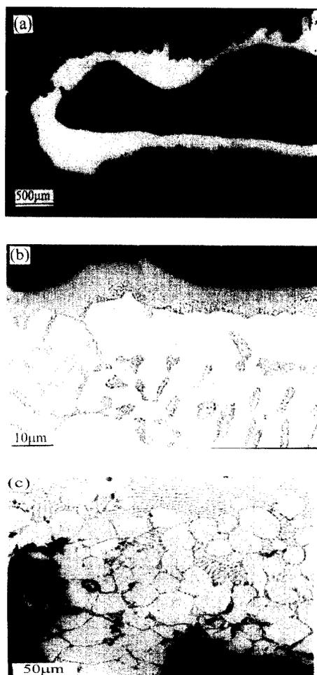
**Fig. 7.** Microstructures of pure Al corroded inside molten  $ZnCl_2$ -KCl salt at 450°C. (a): general view; (b): expanded view between the Al matrix (black) and the external area (light) interface; (c): expanded view of the outmost light region in (a)
