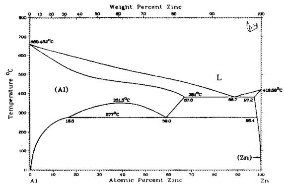
Fig. 9. Phase diagram of binary Al-Zn system
