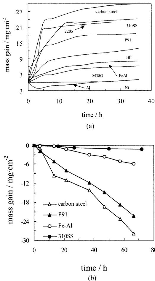
Fig. 2. Corrosion kinetics of examined materials beneath  $ZnCl_2$ -KCl deposit (a) and in molten  $ZnCl_2$ -KCl mixture by immersion test (b) at  $450^\circ C$
