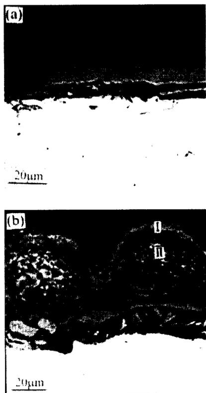
**Fig. 4.** Cross-sectional morphologies of pure Ni (a) and Fe-25Cr (b) corroded beneath KCl deposit at 450°C. (c): EDX results in (b)
