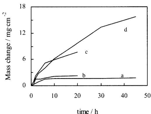
Fig. 3. Corrosion kinetics of carbon steel (a,d) and 310SS (b,c) with (a,b) or without (c,d) aluminized coating beneath KCl deposit at  $650^\circ C$
