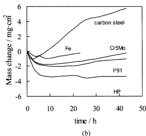
**Fig. 1.** Corrosion kinetics of examined materials beneath KCl (a) and ZnCl<sub>2</sub> (b) deposit at 450°C
