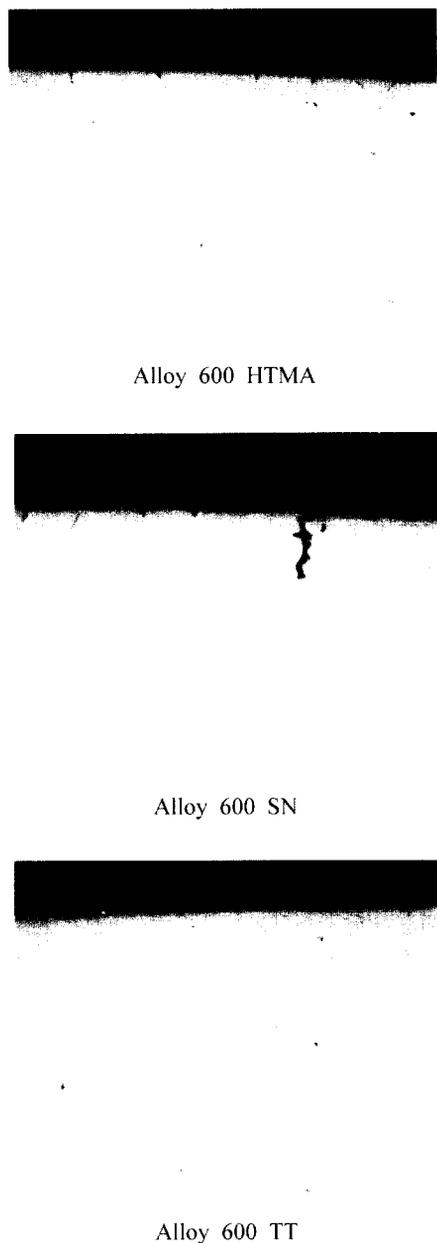
**Fig. 6.** Cross sectional area of C-ring specimen of Alloy 600 at an initial stress of 340 MPa exposed to 0.1 M NaHSO<sub>4</sub> 34 days.
