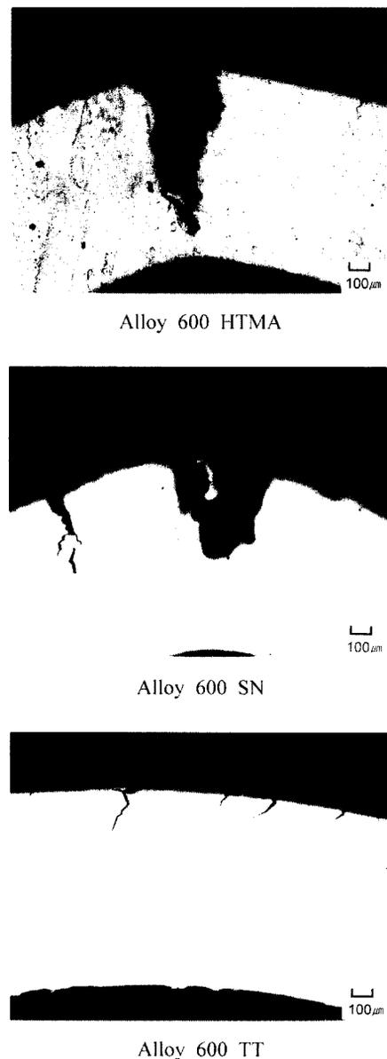
**Fig. 7.** Cross sectional area of C-ring specimen of Alloy 600 at an initial stress of 565 MPa exposed to 10 % NaOH for 9 days.
