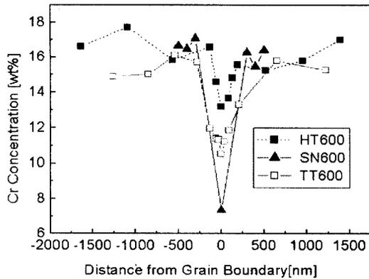
Fig. 4. Cr concentration profiles across the grain boundaries of the Alloy 600s
