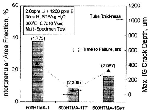
Fig. 5. Susceptibility to PWSCC of the Alloy 600s
