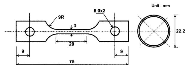
**Fig. 1.** The shape and dimensions of the CERT specimen used in this study.
