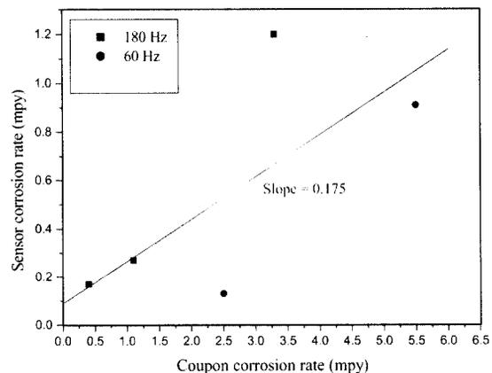
Fig. 10. The corrosion ratio of the sensor corrosion rate to coupon corrosion rate
