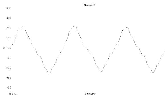
Fig. 5. Typical Pipe-to-Soil Potential Profile (Vertical grid: 10V, Horizontal grid 5msec.)
