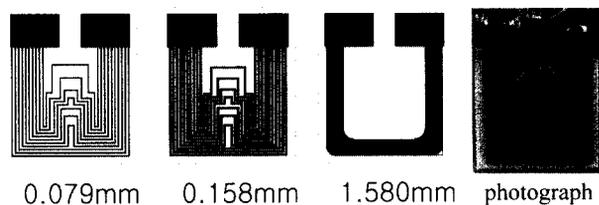
**Fig. 2.** The Shape of Thin Film Electric Resistance Sensor
