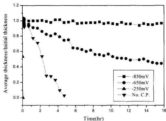
Fig. 4. The corrosion rate change with the cathodic protection potential (solution resistivity: 100 Ωcm, NaCl aqueous solution)
