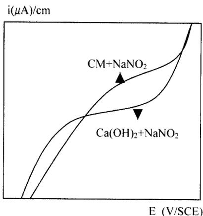
**Fig. 1.** Polarization curves of mild steel in cement extract and Ca(OH)<sub>2</sub> in the presence of 0.2% sodium nitrite
