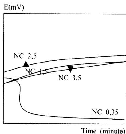
**Fig. 2.** Corrosion potential-time curves with different concentrations of calcium nitrite (NC) inhibitor
