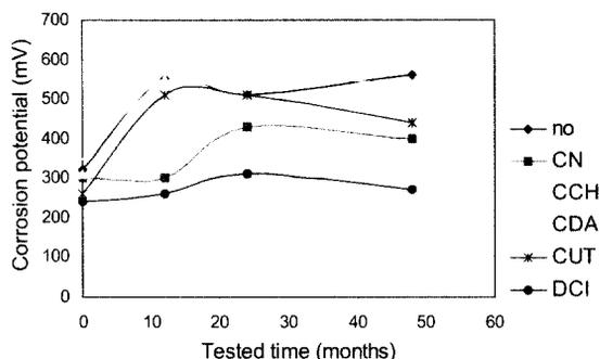
Fig. 3. The change of corrosion potential in CuaLo Tests
