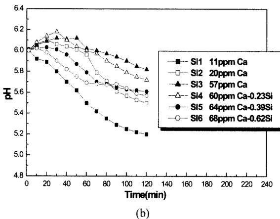
Fig. 2. Change in pH value of thin water film measured for 2 hours at room temperature using a micro-pH electrode (a) in distilled water (b) in a 0.1M NaCl solution. The water film thickness was 2mm.
