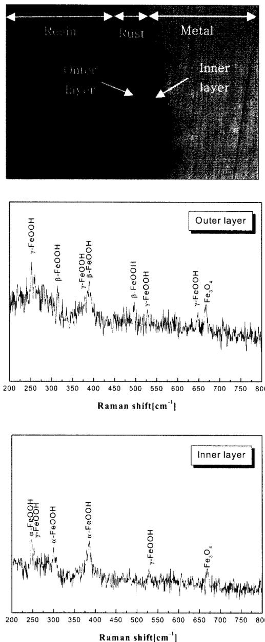
Fig. 4. Image and phase identification by Raman analysis across the rust layer formed on the SI5 specimen over 480 cycles in the cyclic corrosion tester.
