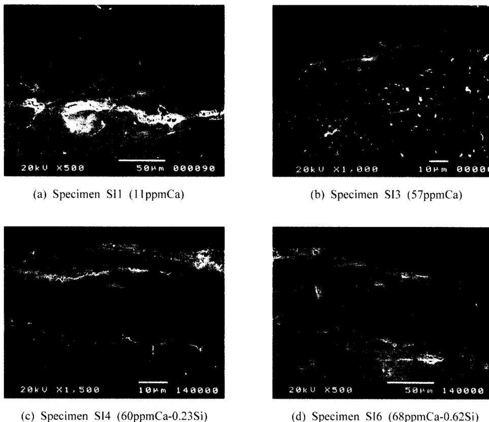
Fig. 5. Cross-sectional morphologies of rust layers formed on the surface of specimens corroded during 480 cycles in the cyclic corrosion tester.
