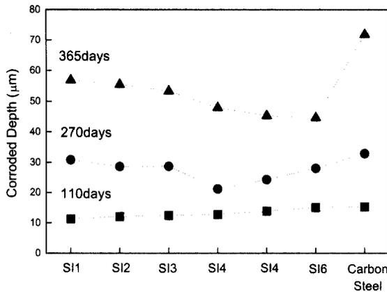
Fig. 6. Change in corrosion depth of the steel specimens during atmospheric exposure in a marine environment.
