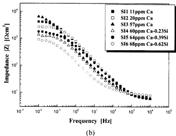
Fig. 3. Bode plots of AC impedance data for the specimens covered with a thin water film of (a) 0.01M NaCl solution (b) 0.1M NaCl solution
