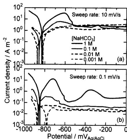
Fig. 9. Polarization curves measured at two scan rate for decarburized SM400B carbon steel in NaHCO<sub>3</sub> solution as a function of concentration of NaHCO<sub>3</sub>.
