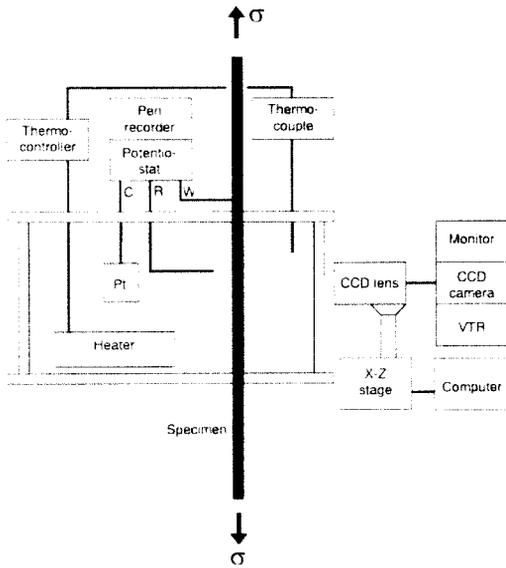
Fig. 1. Schematic illustration of a slow strain rate testing apparatus with dynamic observation system.
