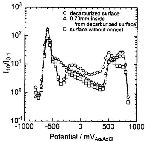
Fig. 8. Ratio of current densities measured at two scan rates plotted against potential from Fig. 7.
