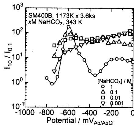
Fig. 10. Ratio of current densities measured at two scan rates plotted against potential from Fig. 9.
