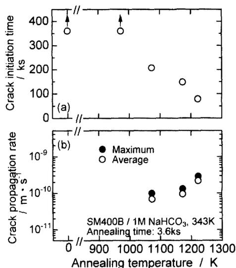
**Fig. 3.** Effect of annealing temperature on (a) crack initiation time and (b) crack propagation rate for SM400B carbon steel in 1M NaHCO<sub>3</sub> at -600 mV.
