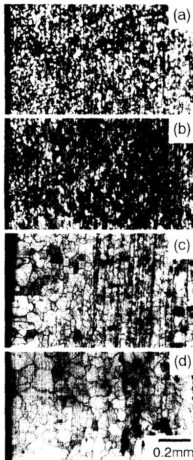
**Fig. 4.** Change in microstructure of SM400B carbon steel with annealing temperature. (a) as-received, (b) 973, (c) 1173, and (d) 1223 K
