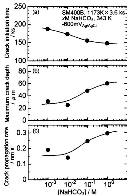
**Fig. 6.** Effect of concentration of  $\text{NaHCO}_3$  on (a) crack initiation time, (b) maximum crack depth and (c) maximum crack propagation rate for annealed SM400B carbon steel in  $\text{NaHCO}_3$  solutions.
