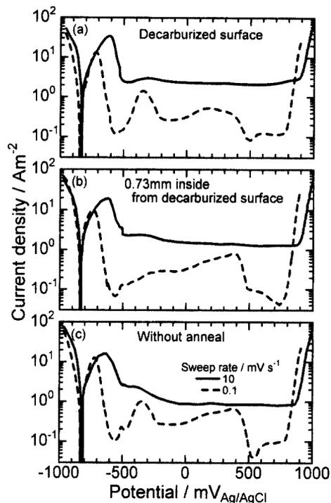
Fig. 7. Polarization curves measured at two scan rate for (a) decarburized surface, (b) the surface 0.73 mm inside from decarburized layer, and (c) the surface of non-annealed SM400B carbon steel in 1 M NaHCO<sub>3</sub> solution.
