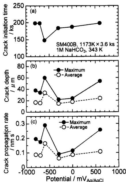
**Fig. 5.** Effect of applied potential on (a) crack initiation time, (b) crack depth and (c) crack propagation rate for annealed SM400B carbon steel in 1 M  $\text{NaHCO}_3$  solution.
