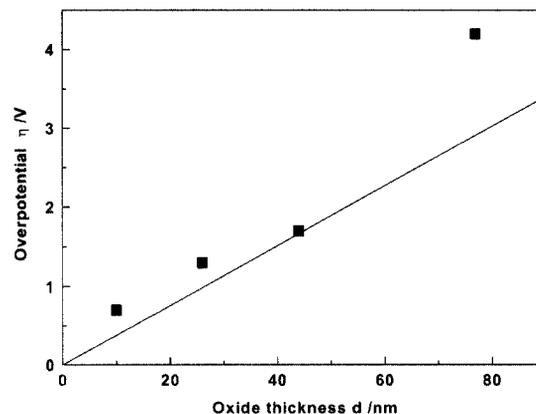
Fig. 3. Overpotential  $\eta$  in the oxide film as a function of oxide film thickness  $d$ .
