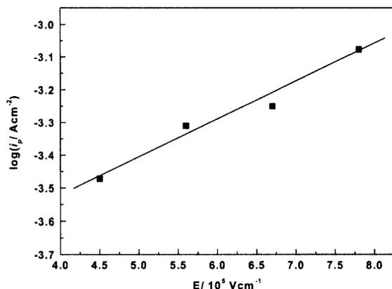
Fig. 5. Plot representing variation of proton transport current density  $i_p$  with electric field strength  $E$  in the film ( $i_p$  is calculated from ERDA)
