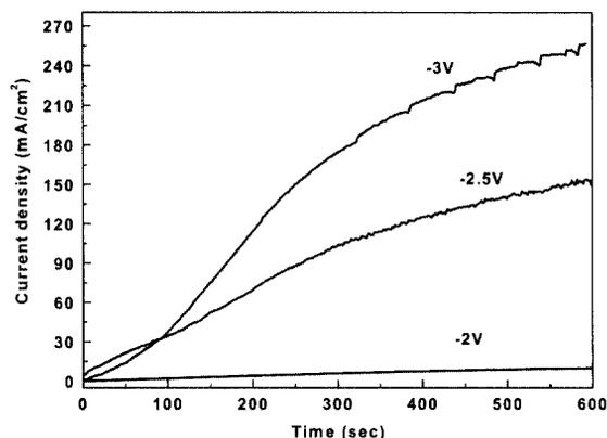
Fig. 2. Hydrogen reduction current of 40 nm thick oxide covered aluminum with different cathodic potentials in 1M HCl solution at 30°C
