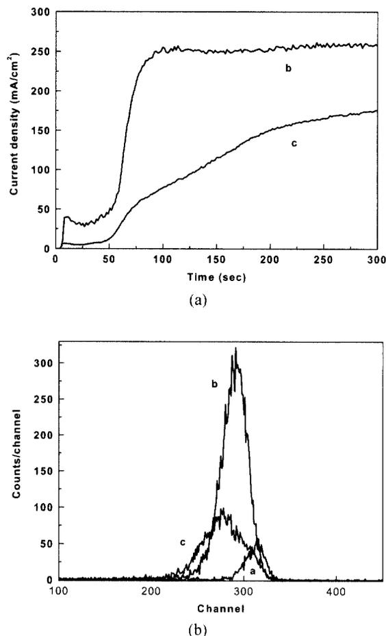
**Fig. 4.** (a) Hydrogen evolution current transient curves of anodized aluminum in 1M HCl polarized at -3V for 300sec, curve b 20 nm thick oxide and curve c 35 nm thick oxide; (b) corresponding ERDA spectra for curve a 20 nm thick oxide without cathodic polarization, curve b and c were the same condition as in (a).
