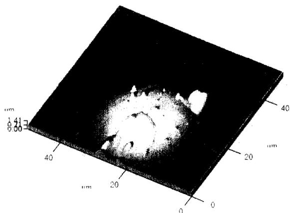
**Fig. 8.** Atomic force micrograph showing blister formed on aluminum surface covered with 40 nm thick oxide film after cathodic polarization at  $-3V$  for 10 s in 1M HCl at  $30^{\circ}C$ .
