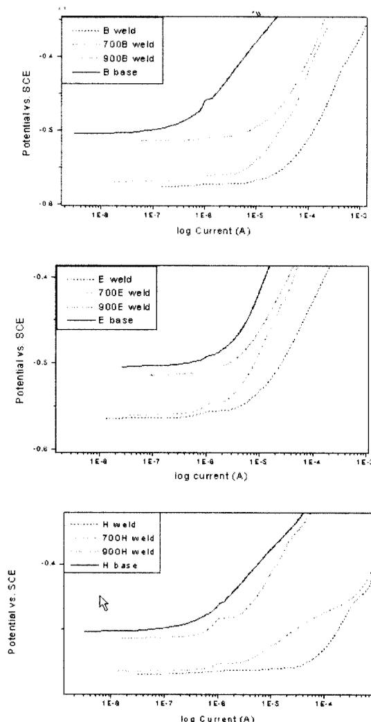
**Fig. 7. Polarization curves of ERW pipes (E,B,H specimen)**
