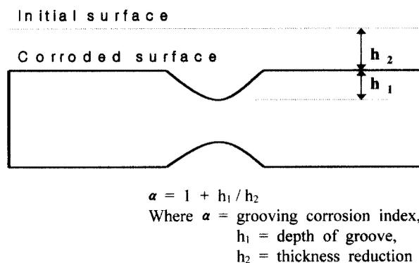
**Fig. 1.** schematic diagram of corroded specimen
